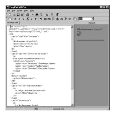
Supporting WML 1.1, WAPPage 2.1 allows the easy creation and maintenance of WML content without users necessarily needing to know too much about WML. WAPPage shows the content in an emulated WAP handset, and you can navigate the WML content by using the built-in tree view. The compiler allows you to quickly locate errors and projects help you group files together. As with many other editors, it features syntax highlighting but also features dragand-drop WML editing.
