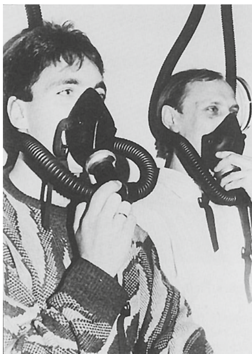
Fig. 7.12 Oxygen masks for use in hyperbaric chambers
