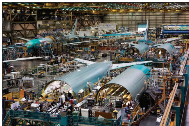
These employees are conducting final assembly of a Boeing 777 airplane in the Everett, Washington, plant. Final assembly can involve between 800 and 1,200 people working to complete subassemblies and to integrate systems. This is a classic example of a modular structure. © Patrick T. Fallon/Bloomberg/Getty Images
