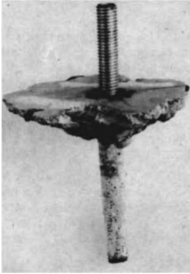
Fig. 6.1 Pulled out chemical fastener with combined pull-out and concrete break-out after a test (Eligehausen, Mallée, and Rehm (1984))
