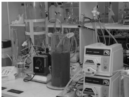
Figure 13.1 (See color insert following page 292.) This figure depicts a potentially dangerous environmental engineering experiment. Air is passed through an aeration tank containing bacterial biomass. The resulting contaminated air contains aerosols of pathogenic and opportunistic microorganisms and must be filtered before being released into the atmosphere.
