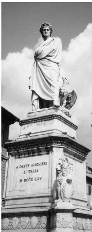
Figure 23.1 (See color insert following page 292.) Biodeterioration caused by sulfate-reducing bacteria on a marble statue (black plumes of CaS).
