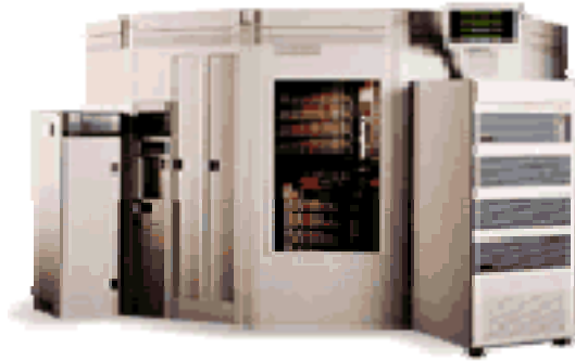
FIGURE 7.6 The StorageTek PowderHorn 9310. This storage silo holds 2000 to 6000 tape cartridges per Library Storage Module (LSM); using the 9840 cartridge, the total uncompressed capacity is 300 terabytes. Each cartridge holds 20 GB of uncompressed data. Depending on the block size and compression, reader transfer at 1.6 to 7.7 MB/second in tests, with a peak speed of 20 MB/second of compressed data. Each LSM has up to 10 tape readers, and can exchange up to 450 cartridges per hour. One LSM is 7.7 feet tall, 10.7 feet in diameter, uses about 1.1 kilowatts, and weighs 8200 pounds. Sixteen LSMs can be linked together to pass cartridges between modules, increasing storage capacity another order of magnitude (Courtesy STC.)
