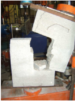
SCC and no TR
