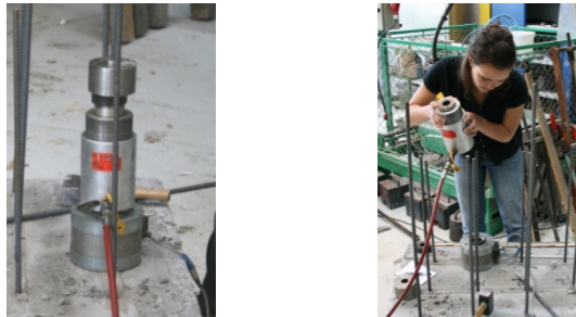
Figure 4. The hydraulic jack setup used for testing the bond strength.
