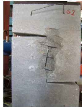
Precracked SCC without TR
