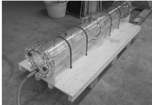
Figure 3. Picture of one of the three sections of the Plexiglas setup.
