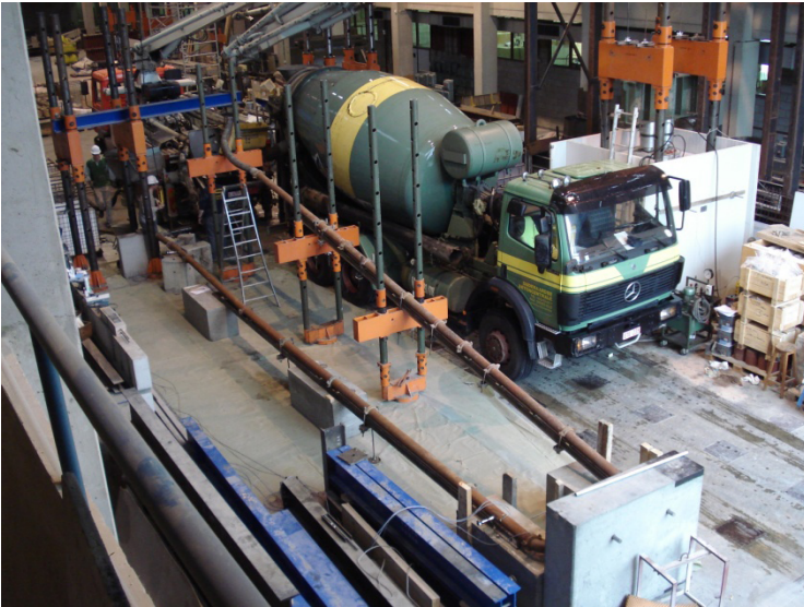
Figure 1. Short pumping circuit (25 m).
