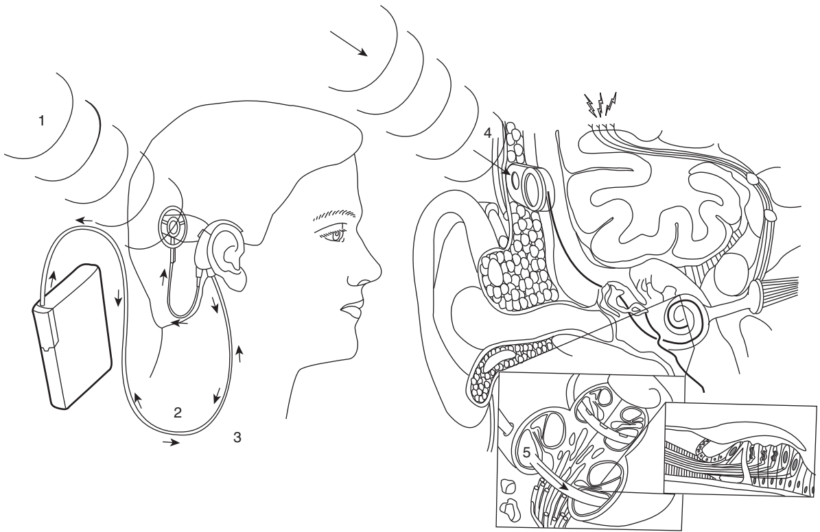
▲ Figure 68-1. Schematic depiction of how cochlear implant systems operate. 1. Sound is detected by an external microphone. 2. This signal is directed to an external sound processor. 3. Once processed, a digital electronic code is sent by a transmitting coil situated over the receiver-stimulator via radiofrequency through the skin. 4. The receiver-stimulator delivers electronic impulses to electrodes on a coil located within the cochlea according to whichever strategy is being used by the processor. 5. Electrodes electrically stimulate spiral ganglion cells and auditory nerve axons.
