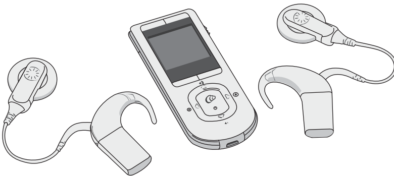
▲ Figure 68-6. The nucleus 5 sound processor with wireless remote assistant for programming. (Image courtesy of the Cochlear Corporation, Sydney, Australia.)
