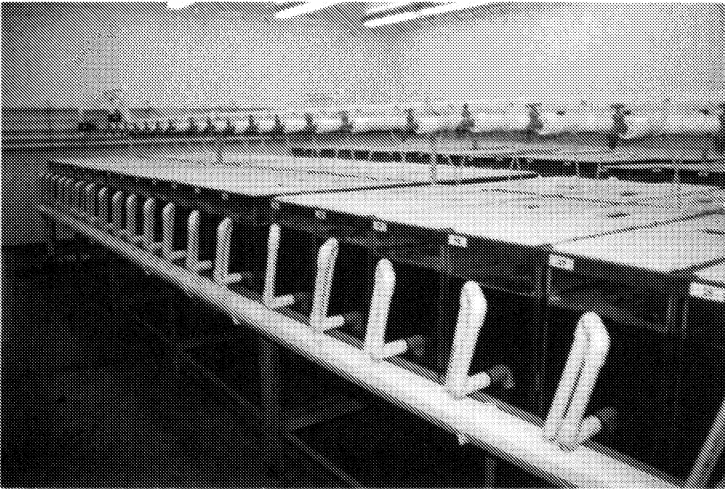
Figure 7.1 Experiments to evaluate the basic nutrition of fish must be conducted in a controlled environment like the laboratory above, where the aquariums have a continuous flow of temperature-controlled, nutrient-free water with sufficient dissolved oxygen. (Courtesy of Meng H. Li.)
