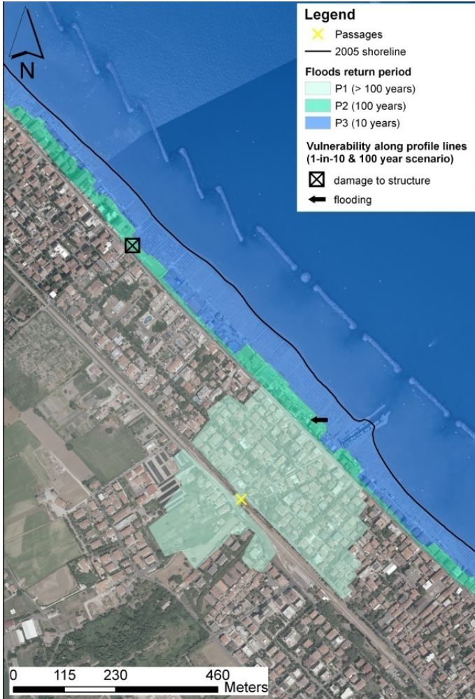
Figure 2.6. Viserba, Rimini province, Italy. Flood hazard map prepared by the Emilia-Romagna Region for marine floods with different return periods. The symbols represent the vulnerability typologies of the 10 and 100 years return period scenarios. The yellow cross represents the location of a low-lying passage which acts as a funnel for inland flooding [PER 16]. For a color version of this figure, see www.iste.co.uk/quevauviller/storms.zip
