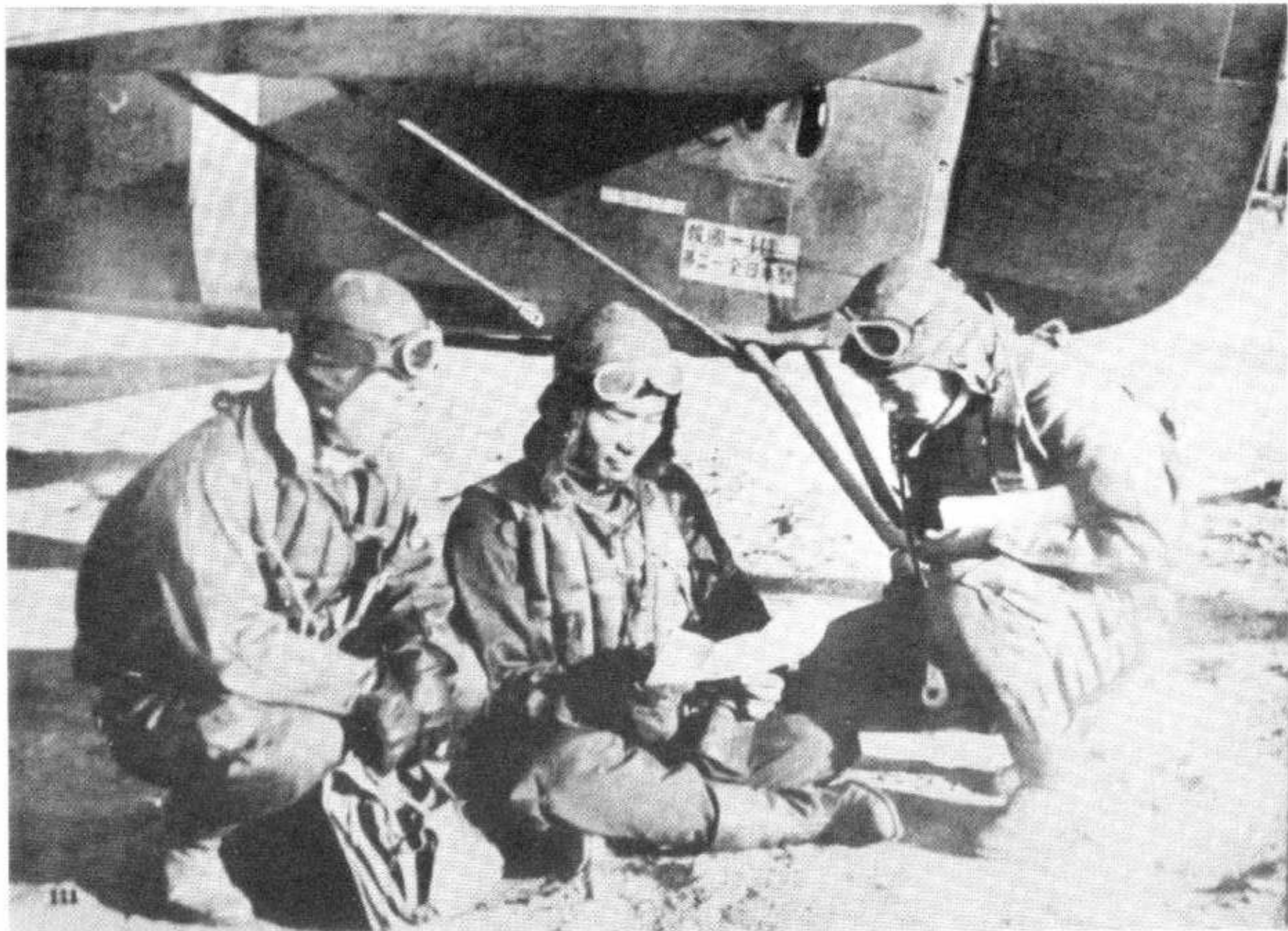
PERRY, showing the early manner of stencilling serial numbers of aircraft. The background color was yellow, black lettering. (J. Wood)
