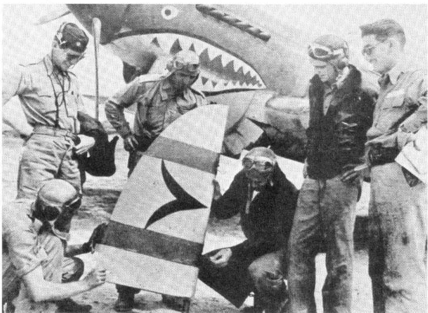
This often published photo of a group of AVG pilots examining the rudder of a fallen NATE of the 2nd Chutai, 77th Fighter Sentai is well worth reprint, if only to demonstrate the typical J.A.A.F. practice of hand-painting the Sentai insignias as opposed to spraying them on. (R. Bueschel)
