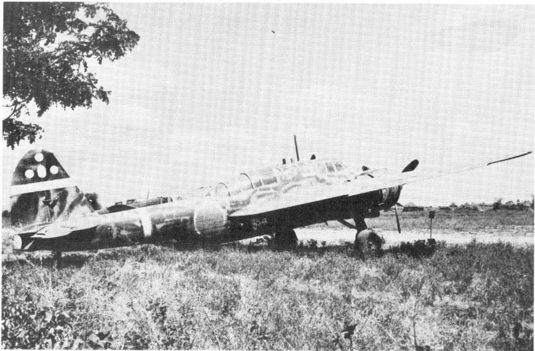
A LILY in a locally applied finish. Note how the dark green has been sprayed around all previous markings, while the newly applied unidentified insignia has been carefully applied over the camouflage coat.
