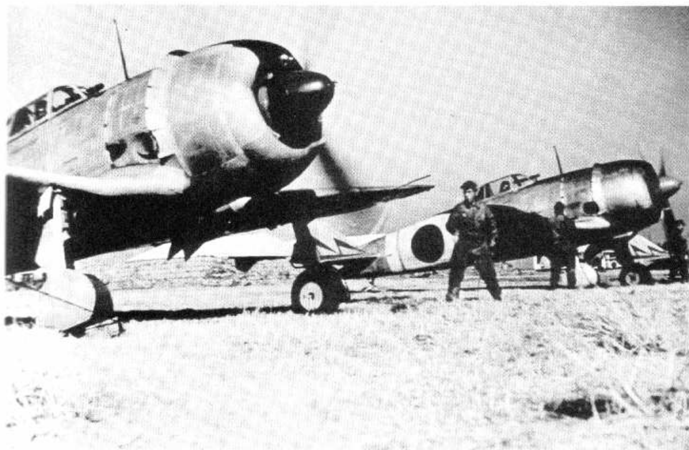
TOJOs of the 47th Fighter Sentai, on Home Defense duties near Tokyo, 1944. Note the unusual application of anti-glare panelling, which was peculiar to this particular aircraft type. (Hideya Anda)
