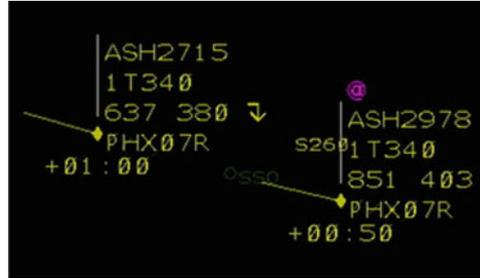
**Fig. 10** FIM aircraft on a radar display [14]: “@” is given to the FIM aircraft
