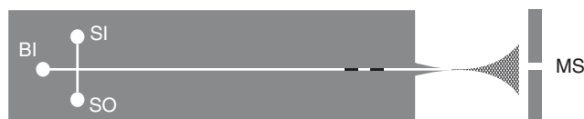
Figure 4.9 Schematic drawing of the MCE device with integrated nanospray emitter. SO, sample outlet; SI, sample inlet; BI, buffer inlet; MS, mass spectrometer. Reproduced from Hoffmann et al. [79] with permission of Wiley.
