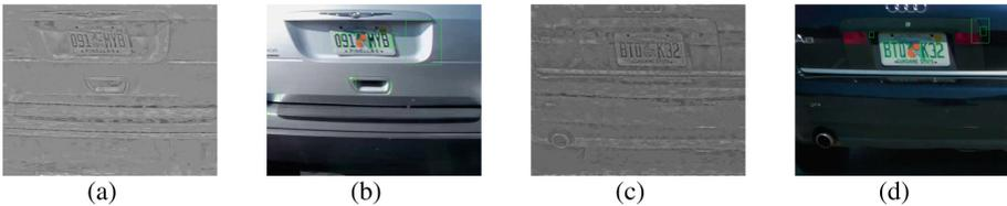
**Fig. 3.** (a) and (c) are the differential images  $G$ ; (b) and (d) are the blobs detected by using MSER on  $G$ .
