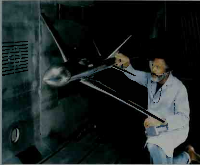
Figure 3.23 Wind tunnels are used to measure the aerodynamic forces on airplane models.
