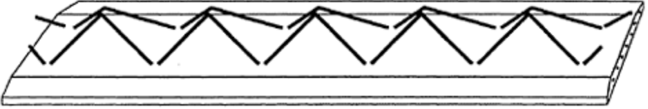
Figure 3 Shows the first phase of the system-producing of flat prestressed polymer modified SFRC plate with needed conventional steel reinforced placed in
