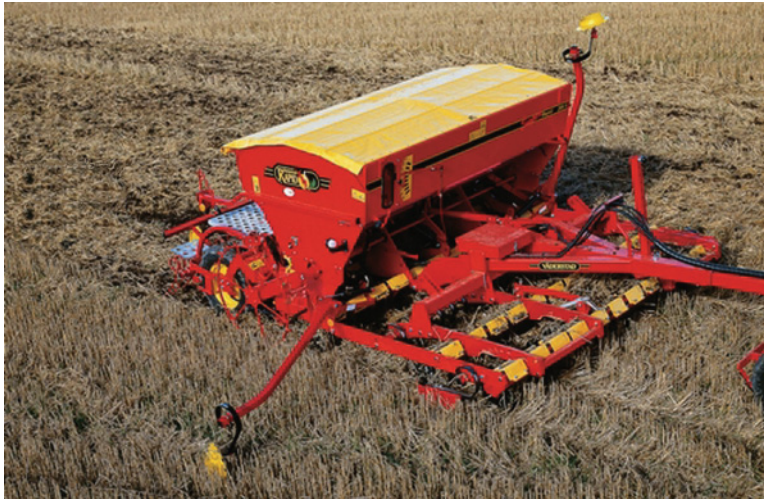
Fig. 9.2. Modern drills can go from stubble to drilled crop in a single pass (photo courtesy of Vaderstad Verken AB).
