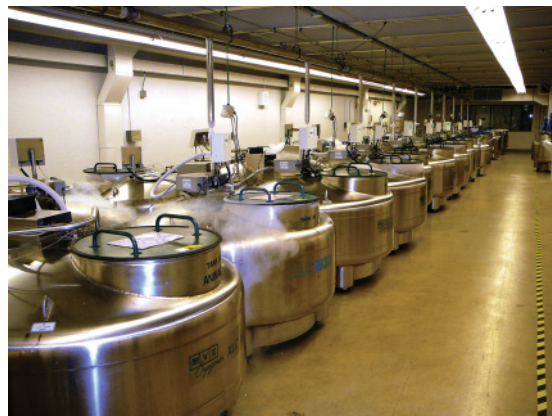
Fig. 7.3. Cryogenic storage tank in the National Center for Genetic Resources Preservation, USDA-ARS, Fort Collins, Colorado, holding safety backup samples of NSGC barley accessions and other germplasm throughout the NPGS. Source: D. Ellis, NCGRP.
