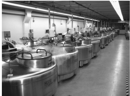
Fig. 7.3. Cryogenic storage tank in the National Center for Genetic Resources Preservation, USDA-ARS, Fort Collins, Colorado, holding safety backup samples of NSGC barley accessions and other germplasm throughout the NPGS. Source: D. Ellis, NCGRP. For color details, please see color plate section.
