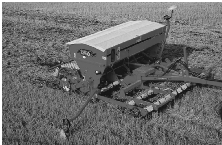
Fig. 9.2. Modern drills can go from stubble to drilled crop in a single pass (photo courtesy of Vaderstad Verken AB). For color details, please see color plate section.
