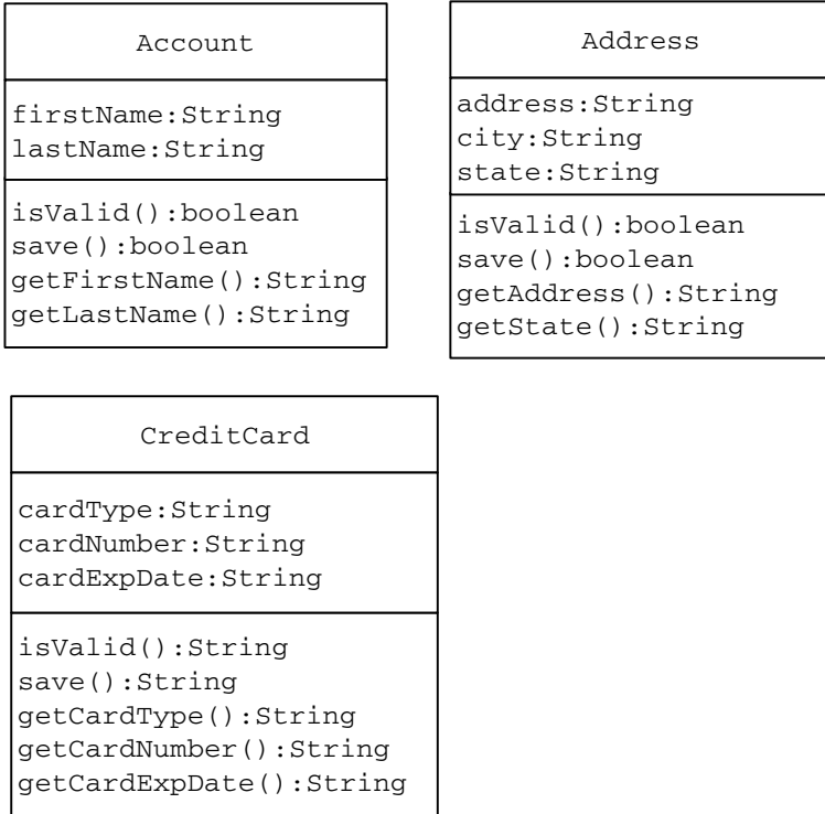
Figure 22.3 Subsystem Classes to Provide the Necessary Functionality to Validate and Save the Customer Data
