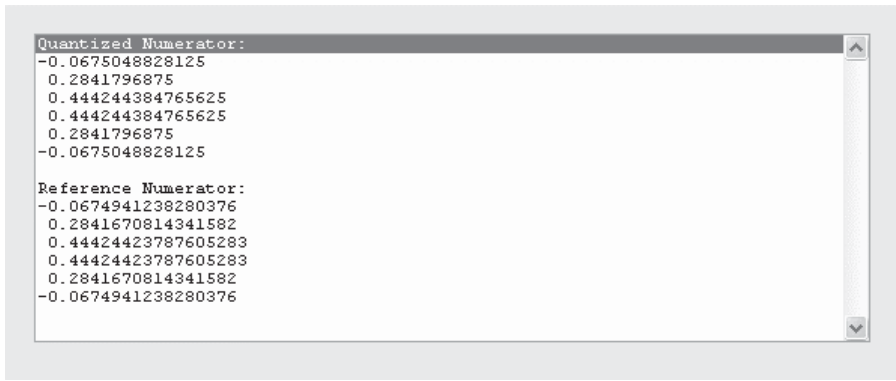
Figure 6.17 Comparison of quantized and reference filter coefficients
