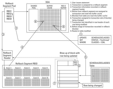
Figure 10-1: Rollback segments and transactions
