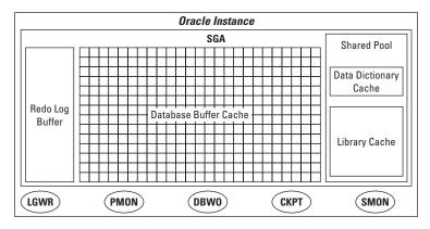
Figure 1-2: The Oracle instance is composed of a number of shared memory areas and background processes.
