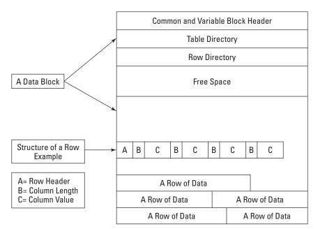
Figure 11-3: Block and row structure
