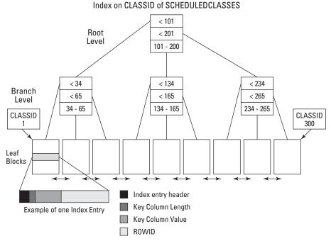
Figure 12-1: Structure of B-tree index
