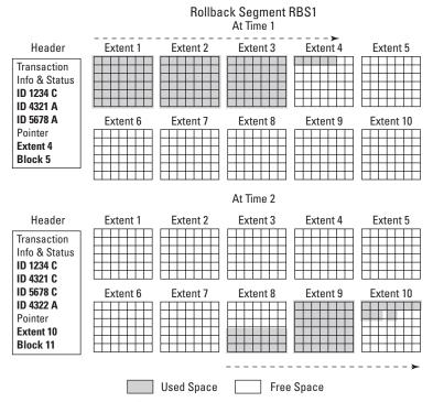
Figure 10-2: How rollback segments use space
