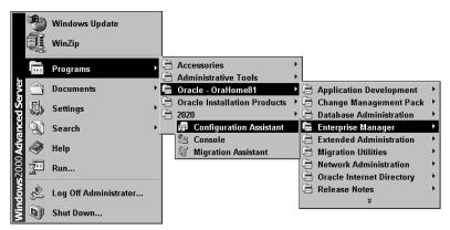
**Figure 2-8:** The Configuration Assistant in the Enterprise Manager program group is used to configure the Oracle Management Server.
