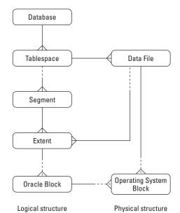
Figure 9-1: The entity relational model of Oracle database storage
