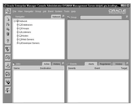
**Figure 2-19:** The main OEM console screen consists of navigator, group (map), job, and event panes.
