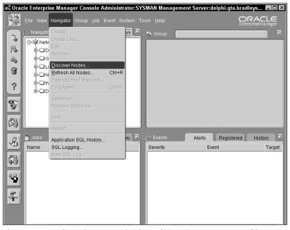
**Figure 2-20:** Select Discover Nodes from the Navigator menu to add databases and other servers to the repository.
