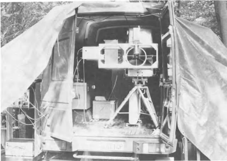
IROE's fluorescence lidar (FLIDAR) at the Garderen field
