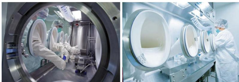
**Fig. 4** Isolator in the ADC GMP large scale production plant at Lonza Ltd, Visp, Switzerland
