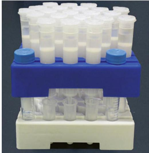
**Fig. 6** Assembled parallel GFC column rack with columns in place. Note that the column outlets are within the tubes to minimize potential static effects. The caps on the columns are normally removed before placing in the rack (not as shown). The upper rack containing the columns nests in the bottom rack containing the collection tubes. The entire assembly including columns is discarded following purification. *See the procedure*
