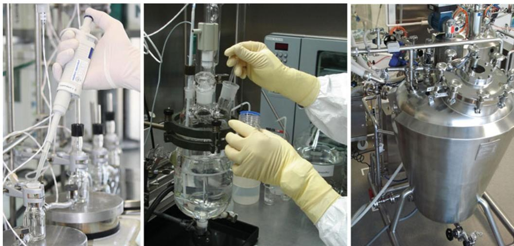
**Fig. 4** ADC process equipment at Lonza Visp: mg-scale jacketed glass reactors, g-scale glass reactor, kg-scale stainless steel reactor
