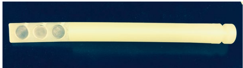
Fig. 8 Image of an individual rod with three biofilm coupons from the CDC biofilm model
