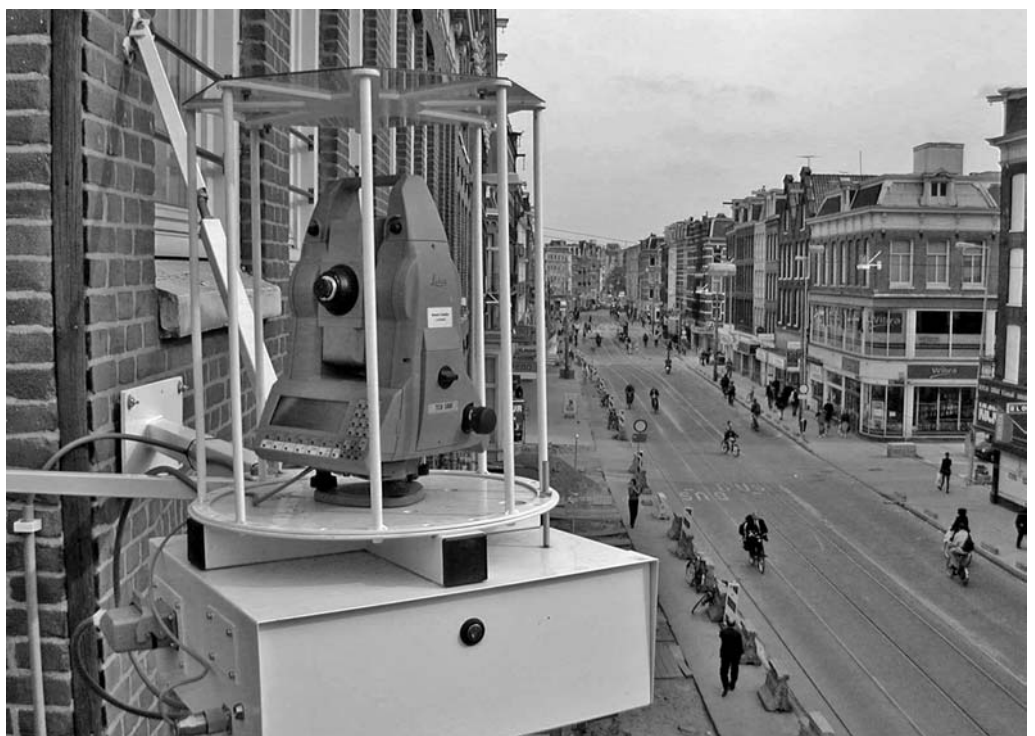
Figure E.1. RTS being used to monitor movements in an urban environment
