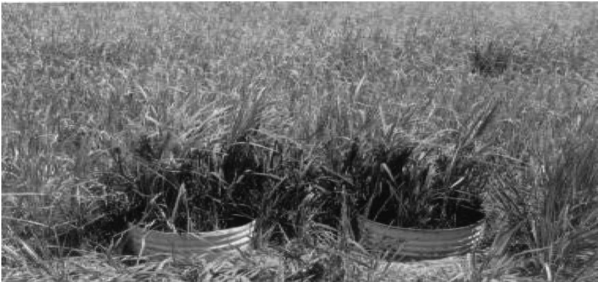
FIGURE 10.3 Drum lysimeter installed in rice field.
