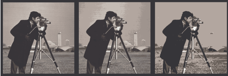
FIGURE 3.4: The effects of an insufficient color depth. Left to right the images use the same resolution and a color depth of 8, 4 and 2 bits/pixel, respectively. Note what happens to the sky in the middle image (4bit/pixel) and to the tower in the background in the image to the right (2 bits/pixel). (Reprinted from Bovik, A., Handbook of Image and Video Processing , 2000, p. 500. With permission from Elsevier Science.)
