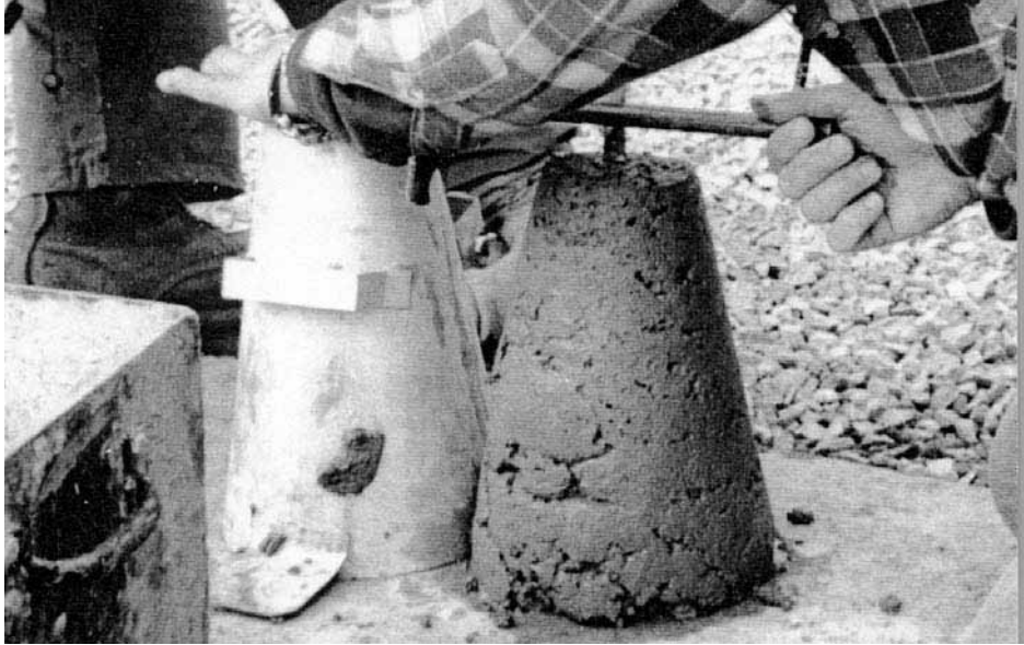
FIGURE 6B.20 ASTM C 143 slump test in progress.
