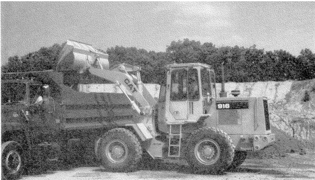
FIGURE 6A.13 Loader dumping soil into a haul truck (courtesy of Caterpillar Inc., Peoria, IL).
