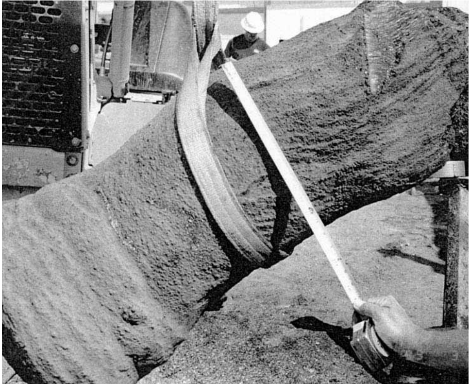
FIGURE 6B.174 Grouted soil mass from a test injection.
