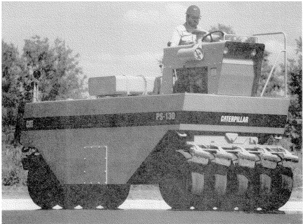
FIGURE 6A.21 Rubber-tired roller (courtesy of Caterpillar Inc., Peoria, IL).
