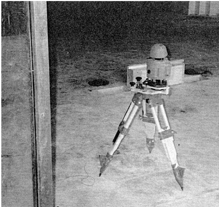
FIGURE 6B.152 The signal from rotating laser instruments can cover a large planar area.
