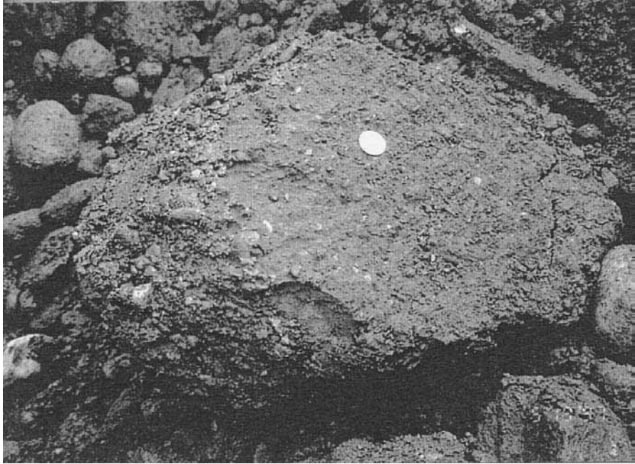
FIGURE 6B.83 Near-perfect columnar mass of grout exposed by excavation of overburden.
