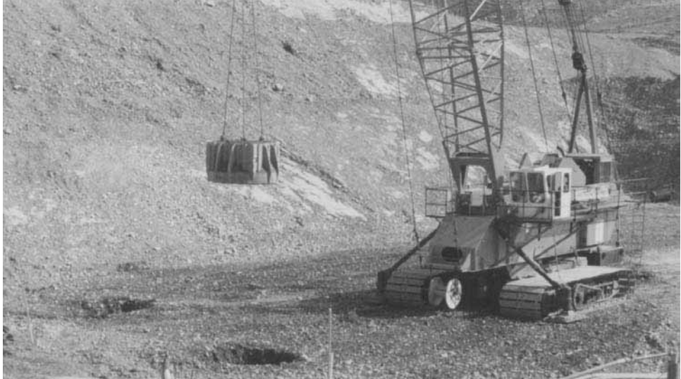
FIGURE 6A.149 Steel tamper with a circular base.
