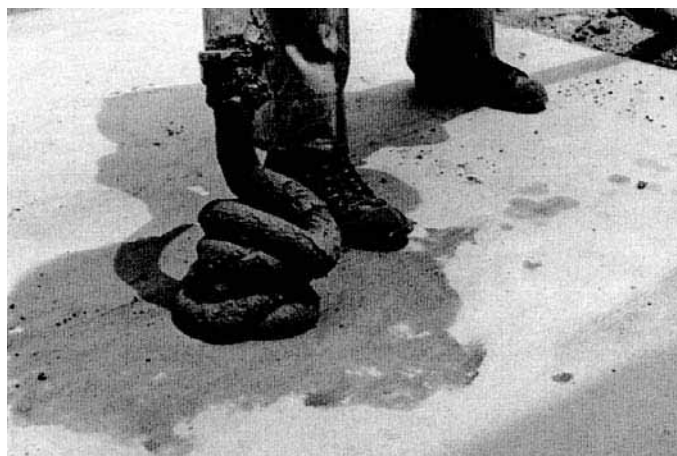
FIGURE 6B.39 Very stiff plastic consistency grout (Warner and Brown, 1974).
