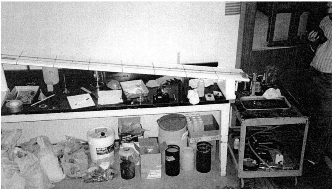
FIGURE 6B.21 Tubing attached to slant board for grout flow evaluation.
