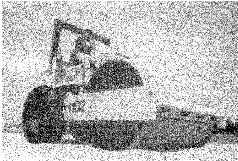
FIGURE 6A.19 Vibratory smooth-drum roller (courtesy of Vibromax 2000 USA Inc., Racine, WI).
