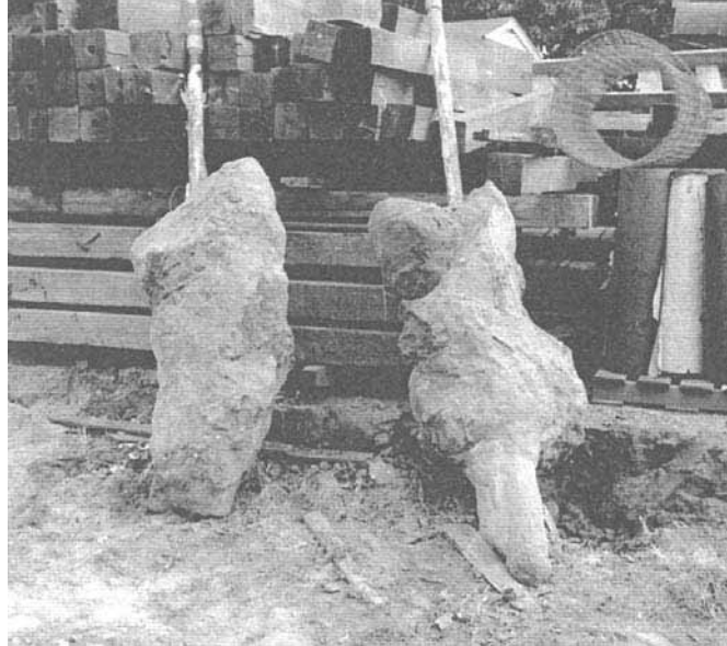
FIGURE 6B.37 Grout “columns” from two test injections (Brown and Warner, 1973).
