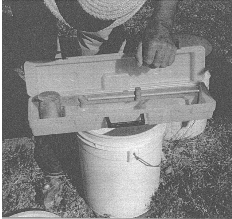
FIGURE 6B.28 Baroid mud balance used for evaluation of grout density.
