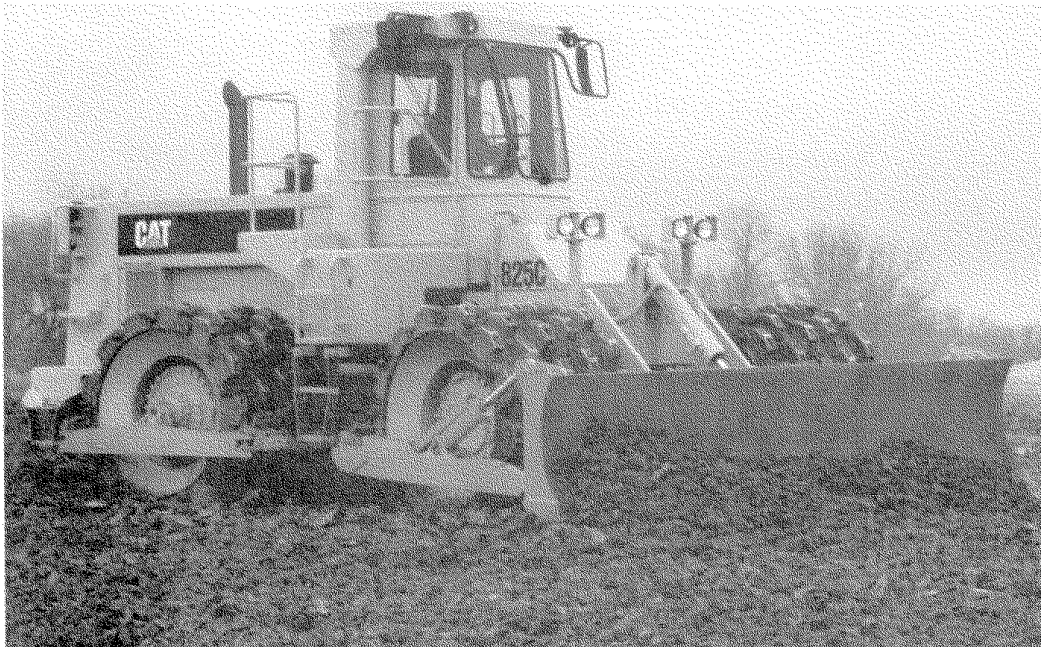
FIGURE 6A.22 Self-propelled tamping foot roller with leveling blade on front (courtesy of Caterpillar Inc., Peoria, IL).
