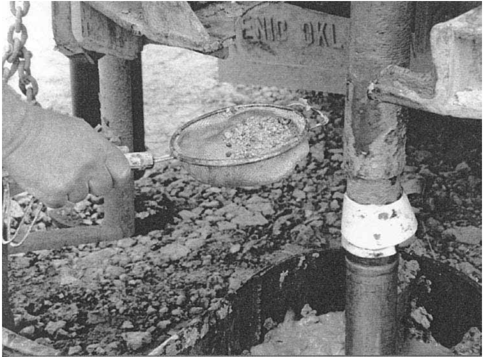
FIGURE 6B.144 Much can be learned from observation of the drill cuttings.
