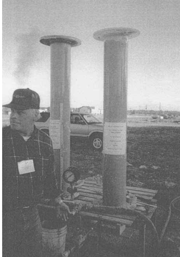
FIGURE 6B.16 Sand-filled columns used to evaluate cement grout penetrability.
