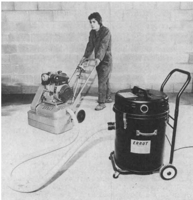
Figure 1 Concrete Grinding Machine with Dust-Extraction Equipment
