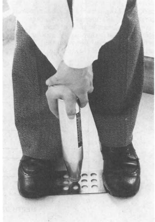
Figure 6 N Type Schmidt Rebound Hammer, (left) Diagrammatic View and (right) Readings being taken through a Positioning Template
