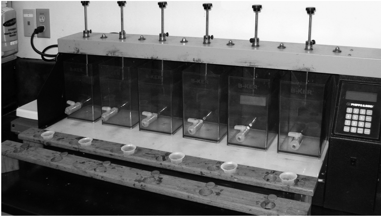
Figure 2-11 Wooden holder for six dosing cups: Small plastic cups fit into each hole drilled in the wood
