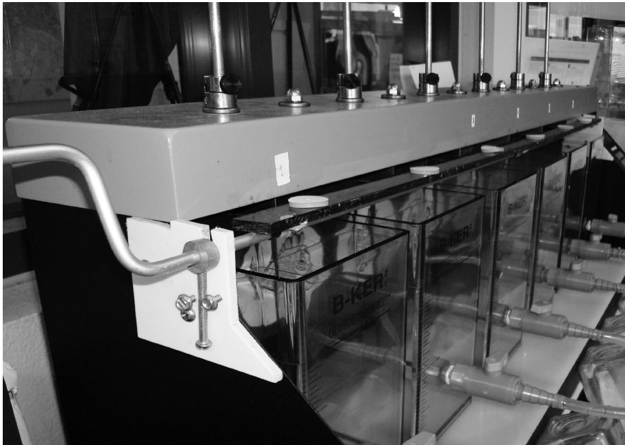
Figure 2-12 Septa bar: Metal bar to hold multiple septa over jars until ready to dump septa into all jars simultaneously.
