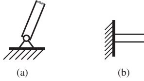
Figure 4: Available boundary conditions: (a) Setting \mathbf{v} = \mathbf{0} on the boundary amounts to a fixed but limp bearing. (b) Enforcing D\mathbf{v}\hat{\mathbf{o}} = \mathbf{0} , where \hat{\mathbf{o}} is the outer normal of \Gamma , suppresses rotations around the boundary curve but does not necessarily limit translational degrees of freedom.
