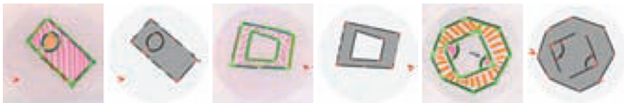
Figure 6: If the design contains a interior room with no exterior walls, this space may be intended as a courtyard space, uncovered by a roof. The system will require extra information from the designer if the default interpretation does not match his/her intentions.
