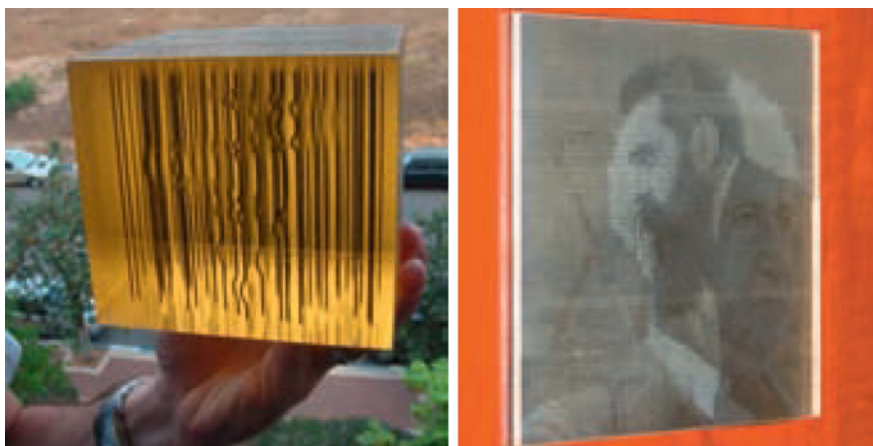
Figure 12: Examples of realized objects from Figures 6 and 9, realized using modern layered manufacturing technology from Object ( www.objet.com ).
