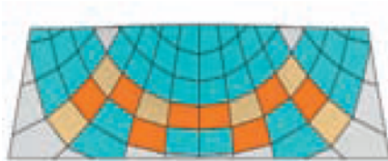
(e) Panels colored by type of corresponding mold.
