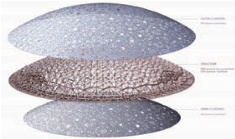
Figure 2: Schematic diagram of the model construction: Structure (middle), cladding layers (top and bottom).
