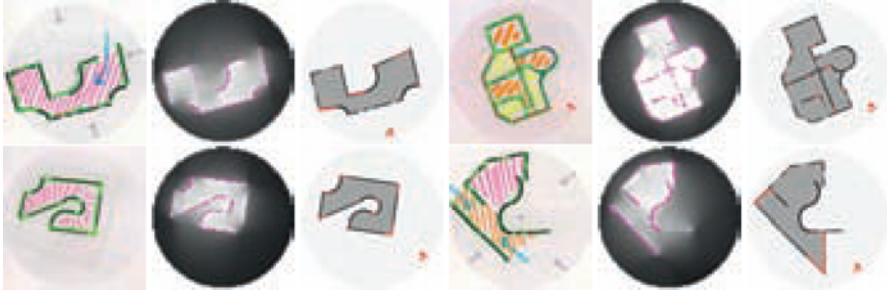
Figure 4: Designs with non convex boundaries may not be accurately extracted with a simple threshold on the average point or cell enclosure. By minimizing the lengths of unused wall and extra inferred wall necessary to enclose the interior zones we correctly interpret these complex designs.
