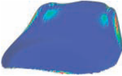
Figure 16: Visualization of Gaussian curvature of the design shown by Figures 11, 12. Blue corresponds to zero, red to the maximum value -0.02 (this means \rho = 7.07 ). The bounding box diagonal of this object is 188.
