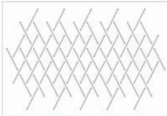
Figure 4. Principal pattern of the Zollinger lamella structure.
