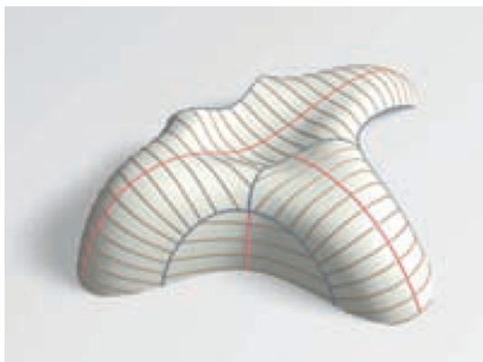
Figure 4: Designing a sequence of geodesics by choosing the locus (red) of minimum distance or maximum distance between neighbours. This is done by the parallel transport method . In this particular example, the method is applied not to the entire surface, but to previously selected patches.
