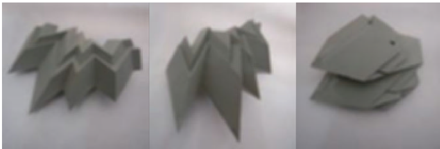
Figure 10: Folded model of a rigid-foldable cylinder. Left: in the developed state, Middle: Intermediate state, Right: flat-folded state.
