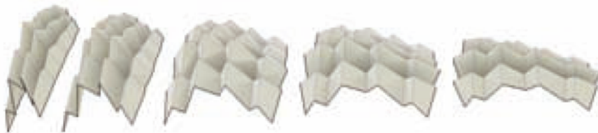
Figure 5: The folding motion of a generalized eggbox pattern.
