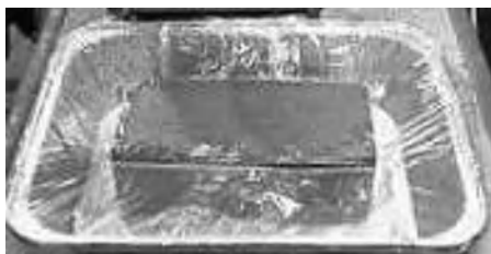
Testing of brick for efflorescence.
