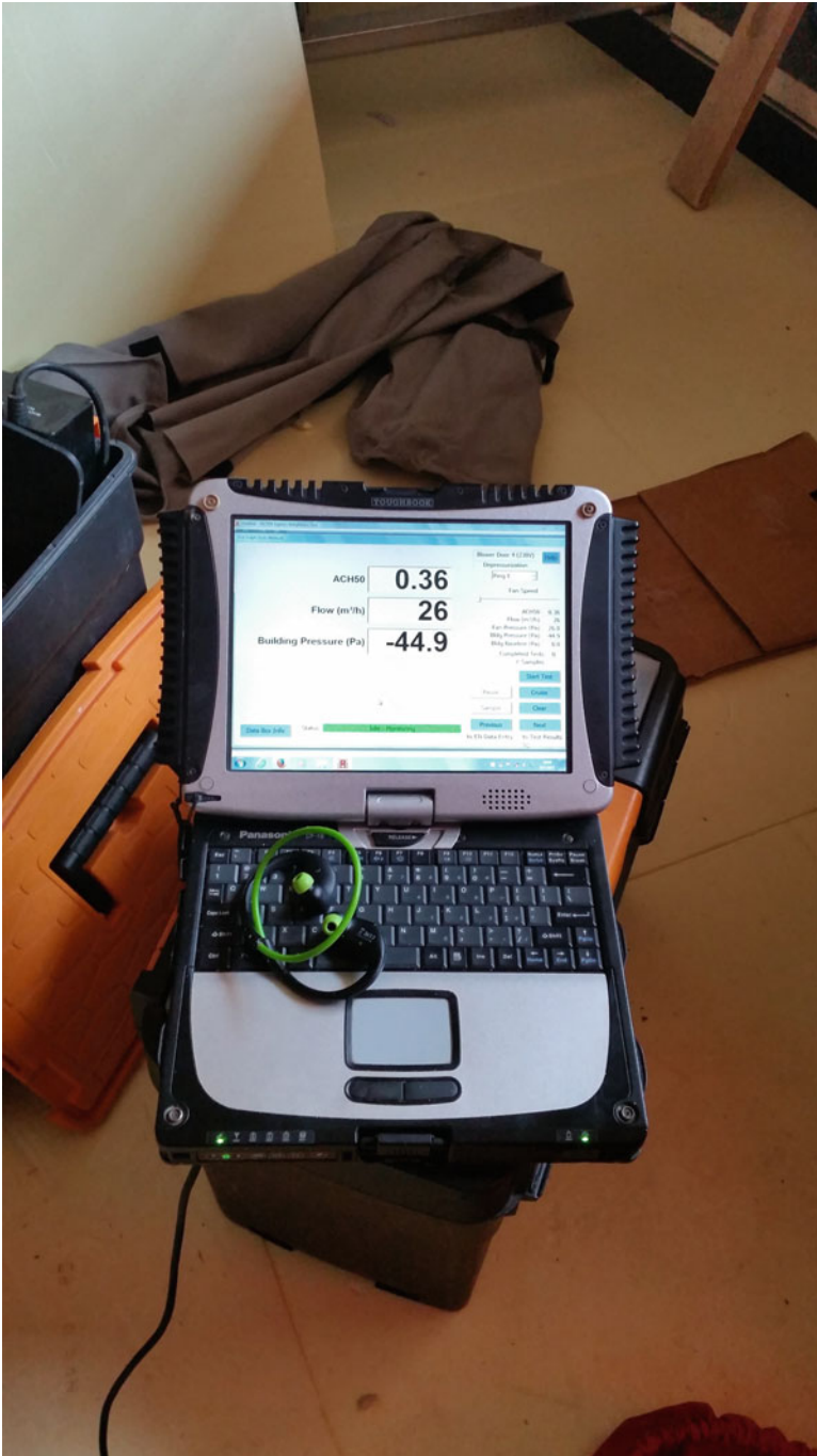
Fig. 8.18 Values detected during the blower door test in vacuum
