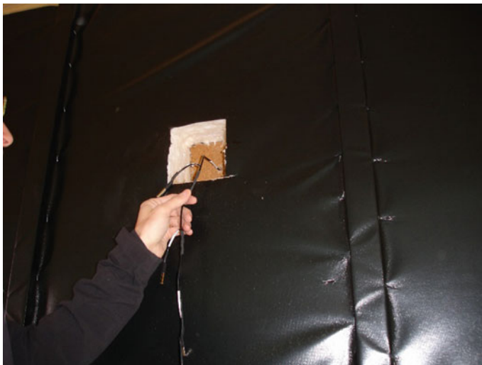
Fig. 10.4 Installation of the wall probe, detail of the contact probes
