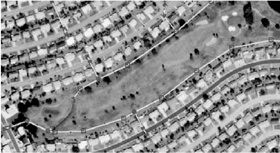
FIGURE 8.2 View of stormwater structures and pipes illustrating topological relationships. (From Landry et al. 2001. With permission.)
