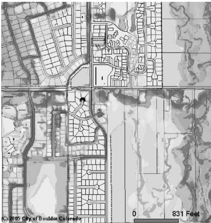
FIGURE 9.8 South Boulder Creek floodplain delineation provides detail on properties and water depths in the regulatory zones. (Source: http://gisweb.ci.boulder.co.us/website/pds/sbc_flood/viewer.htm .)
