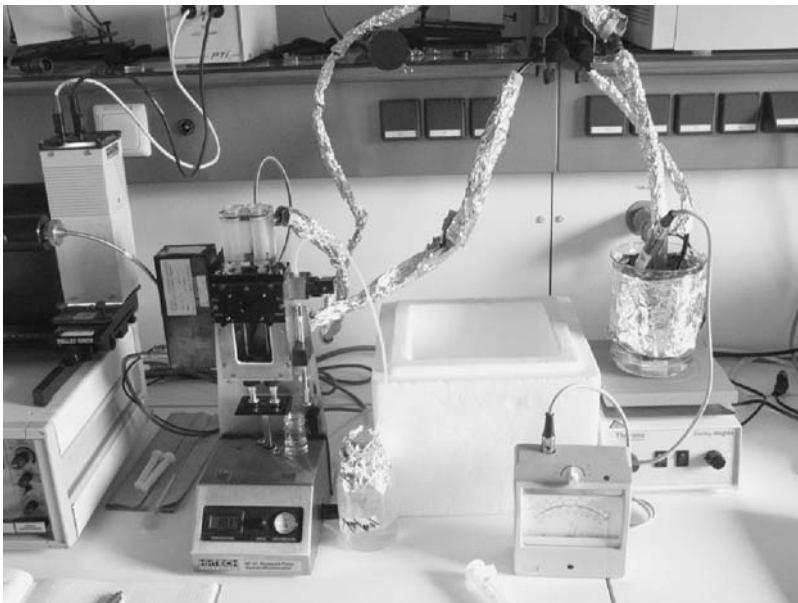
Figure 2 Water circulation at the stopped-flow apparatus. From left to right: electronics unit; sample-handling unit; ice container for cooling and hot plate for heating the circulating solution.
