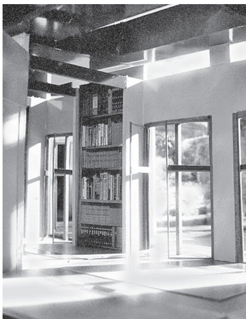
Figure 10.2a A to-scale model of a proposed church interior. One can orient the model to the sun in such a way that would suggest how the actual space might look under the same conditions. But generally, fixed architectural models are representations more than simulations. Courtesy of Professor Matthew Melcher.
