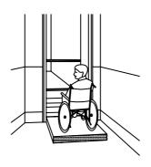
**b** Steps retracted, barrier up, lift starting to rise
