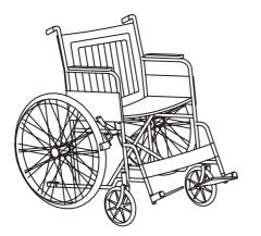
**2.2** Standard wheelchair. For a typical wheelchair of this kind the height above floor level of the top face of the handles is 920 mm and of the top face of the armrests 750 mm
