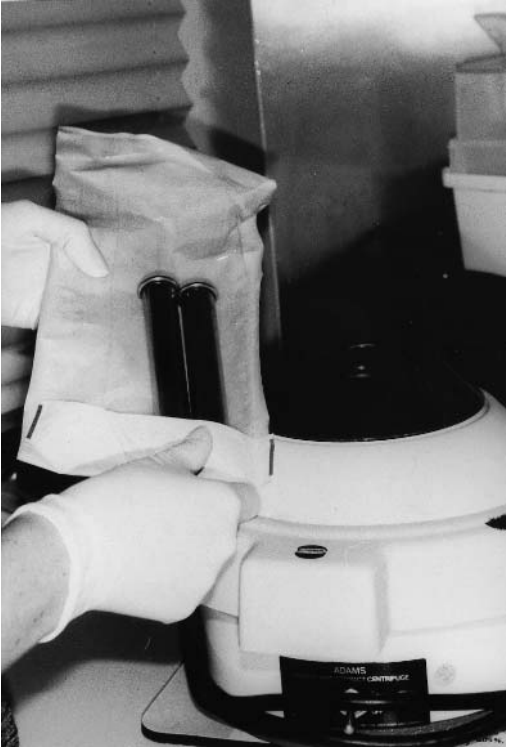
FIGURE 6 Centrifuge with sterilized stainless steel sleeves.
