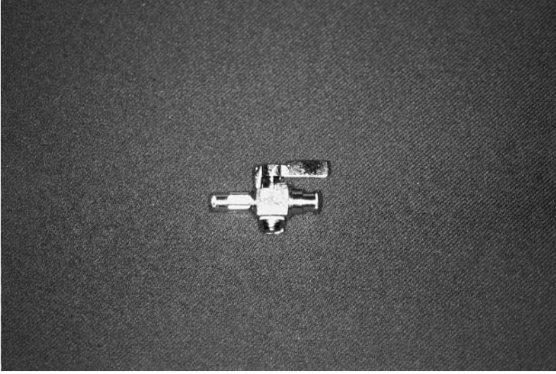
FIGURE 4 Dual luerlock device for processing autologous collagen (Bernsco Surgical Supply, Inc.).
