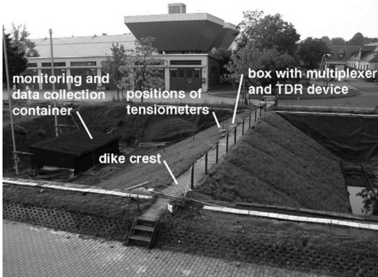
Fig. 1. Full-scale dyke model at the Federal Waterways and Research Institute in Karlsruhe (upstream side on the right)
