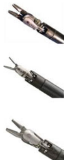
Fig. 17.16 (a–c) EndoWrist instruments (Intuitive Surgical, Sunnyvale, CA) typically utilized in robotic hysterectomy (Modified with permission from Dr. Arnold Advincula, Global Robotic Institute, Florida Hospital, Celebration, FL.)
