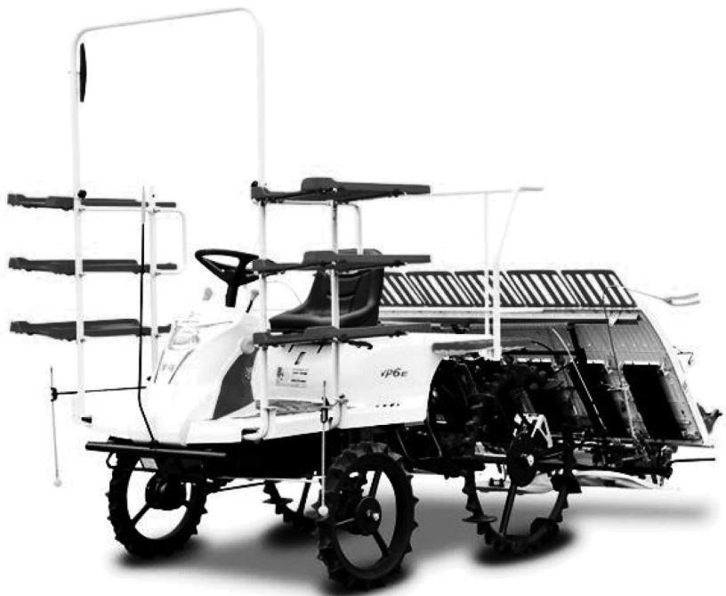
PLATE 2.11 A Semi-autonomous Rice seedling Transplanter [Source: IRRI, Philippines; and Yanmar Agricultural Machinery Manufacturers, Okinawa city, Japan; Note: Robotic Transplanters with GPS connectivity are being developed by a few companies in Japan and other countries in the Tropical Rice Belt. For example, Autonomous Rice transplanter-1-Kubota SPU650 and Iseki PZ60 (see Nagasaka et al., 2010)].
