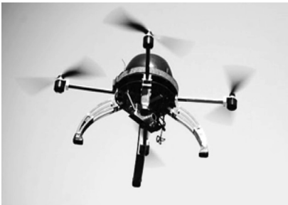
PLATE 3.10 Venture Aerial Robotic Drones- two close-up views in the air (Source: Dr. Rory Paul, Chief Executive Officer, Volt Aerial Robotics Inc., Chesterfield, Missouri, USA. Note: The Quadcopters shown above are highly versatile flying machines with ability to transit at low altitudes above the crop. They could be programed or remote controlled using radio controls. They are effective in obtaining imagery of natural resources, soils and crop stand).
