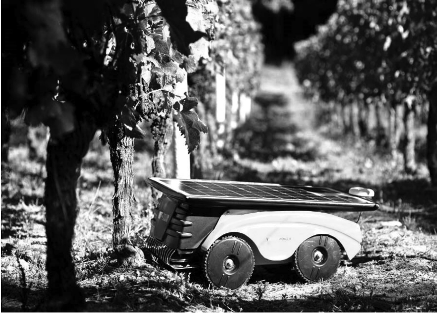
PLATE 2.21 Vitirover – An Autonomous Robot used in Grape vines of Southern France (Source: Dr. Arnaud Frauchdiere, Vitirover, La gare de Saint Emilion, France; http://www.vitirover.com ).
