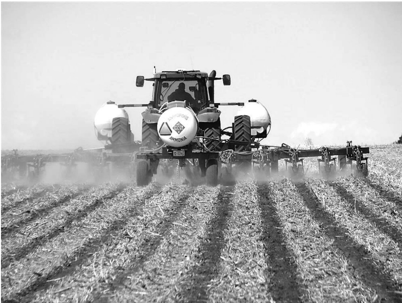
PLATE 4.10 Strip cultivation and variable rate nitrogen fertilizer supply (Note: Strip cultivation is one of the Management Zones concepts adopted as part of Precision Farming. Management zones help in rapid and easier application of fertilizer-N ( \text{NH}_3 ) to soil. Source: Mr. Dean, Twin Diamond Industries, Minden, Nebraska, USA).
