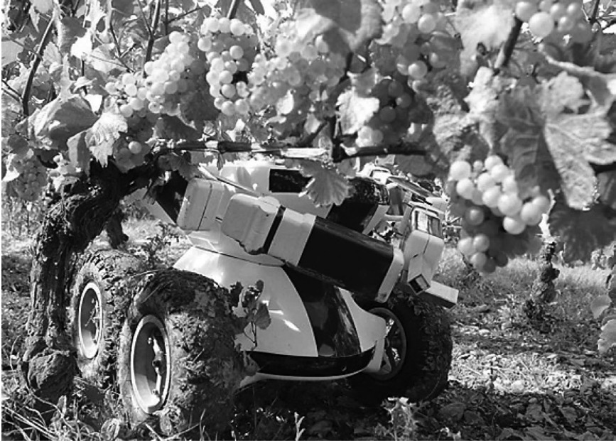
PLATE 2.30 ‘Wall Ye’ A grapevine harvesting robot in operation in a French Grape Farm (Source: Dr. Christophe Millot- Inventor and Dr. Guy Julian- Manufacturer; http://www.kare11.com/video/1860715174001/1/wall-Ye-Wine-Robot-takes-bow-in-Burgandy (June, 23 rd , 2014)).
