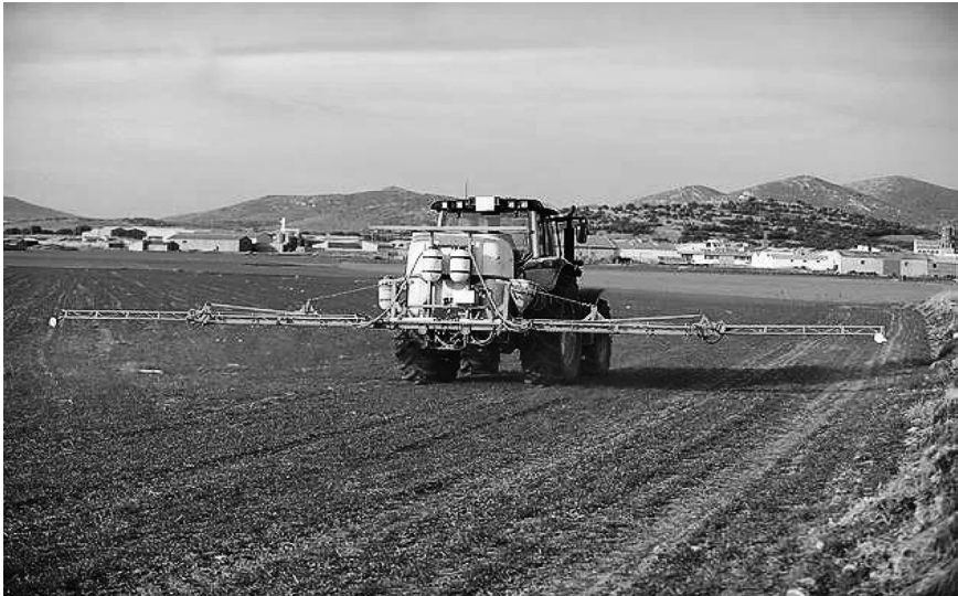
PLATE 2.16 A Semi-autonomous Tractor driven Pesticide Spray System in Western Illinois, USA (Source: Ag Armour Inc., Washington, Illinois, USA).
