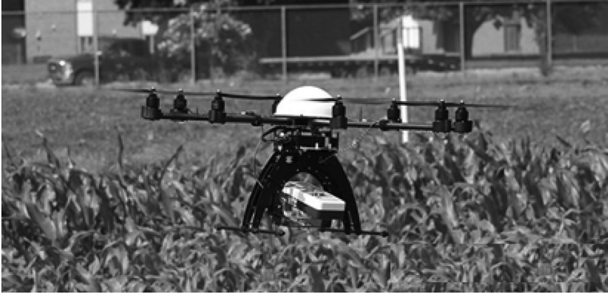
PLATE 3.12B The Hexacopter flying at low altitude above a Maize field (Source: Dr. Rory Paul, Volt Aerial Robotics, Chesterfield, Missouri, USA; Note: These copters have sensors that pick images both at visible and near Infra-Red range. They fly very close to crop to collect images of crop, its growth, chlorophyll content of leaves, disease and pest occurrence, if any.).
