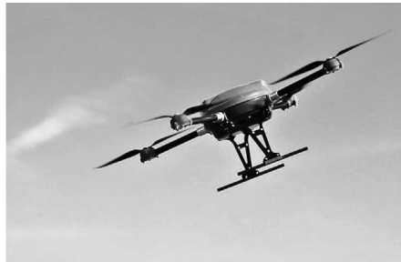
PLATE 3.10 Venture Aerial Robotic Drones- two close-up views in the air (Source: Dr. Rory Paul, Chief Executive Officer, Volt Aerial Robotics Inc., Chesterfield, Missouri, USA. Note: The Quadcopters shown above are highly versatile flying machines with ability to transit at low altitudes above the crop. They could be programed or remote controlled using radio controls. They are effective in obtaining imagery of natural resources, soils and crop stand).
