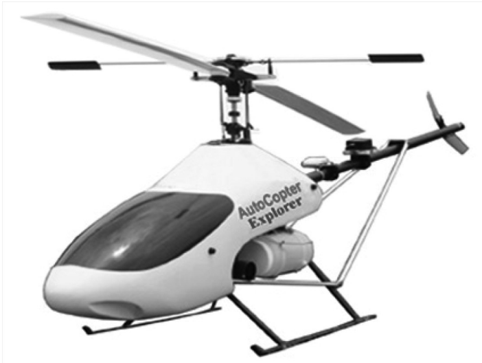
PLATE 3.8B An Autocopter (Source: Dr. Donald Effren, President, Autocopter Inc., North Carolina, USA; Note: Autocopters are used to scout and make aerial imagery of farms and also spray fields with fertilizers/pesticides).
