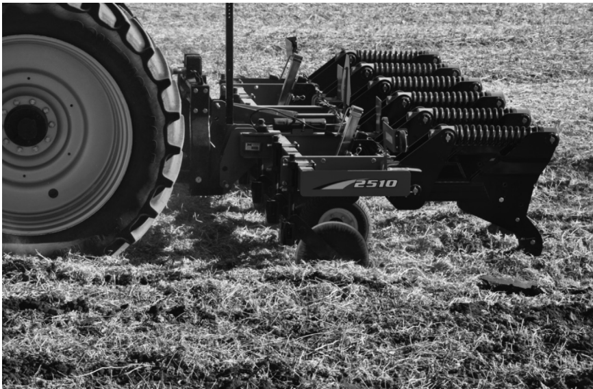
PLATE 2.1 The Landoll 2510 Series In-Row Ripper (Source: Paula-Landoll-Smith, Landoll Corporation, Marysville, Kansas, USA; Note: In-Row rippers are excellent implements for use under Conservation tillage systems. They are good on hard soils that need to be disturbed and turned. Several variations of such rippers are in use for the past 6–8 decades).
