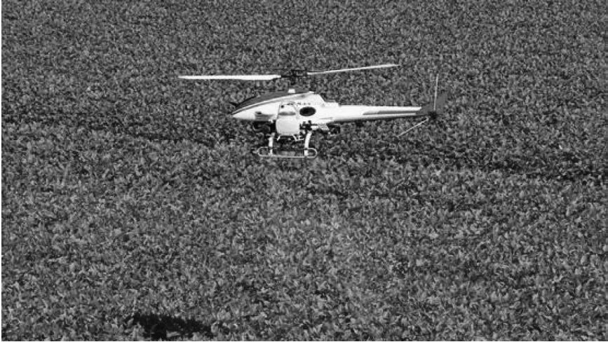
PLATE 3.9 Yamaha RMAX Drone (Note: RMAX is a popular drone among Japanese Agriculturists. RMAX flying at low altitude over a soybean crop. It is spraying pesticide on the crop. Source: Yamaha Motor Co, Australia, http://rmax.yamaha-motor.com.au/agricultural-use ; Barnard Microsystems Inc., http://global.yamaha-motor.com/about/business/sky/ ).
