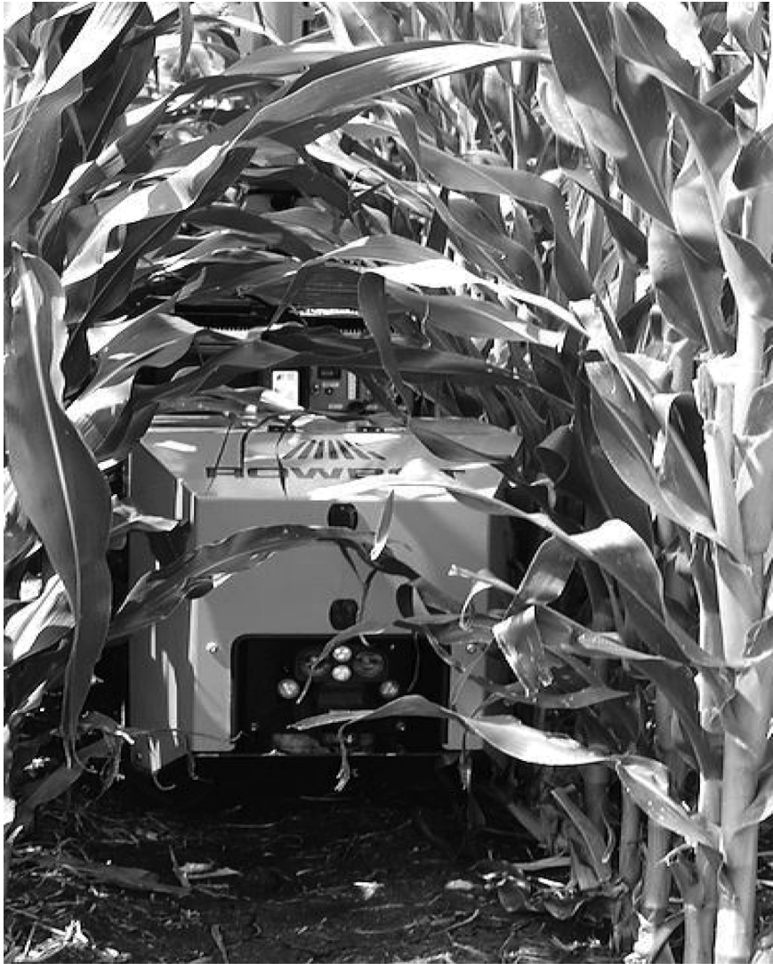
PLATE 2.13 Rowbot's Robotic Fertilizer Applicator (Source: Drs. John Bares and Kent Cavender-Bares, Rowbot, Pittsburgh, Pennsylvania, USA).
