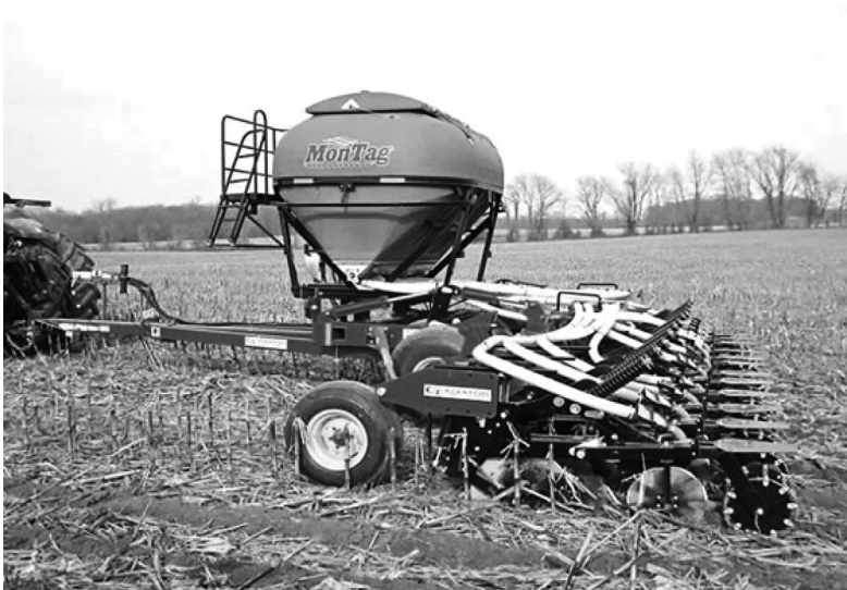
PLATE 4.11A–D A variable rate applicator set for fertilizer supply based on digital maps and satellite guidance (Plate 4.11A: Tractor in front is GPS connected and is hitched to a Variable-rate attachment. Plate 4.11B: The Variable rate fertilizer Nitrogen supplier. The tracks and chains offer better grip and movement. Plate 4.11C: A close-up view of Variable-Rate Applicator. Plate 4.11D: Lateral view of Variable-rate fertilizer N applicator. Note that storage drum is connected to nozzles that are regulated by computer decision support systems. Source: Dr. Rebecca Montag, Vice President, Montag Manufacturing Inc., Emmetsburg, Iowa, USA).
