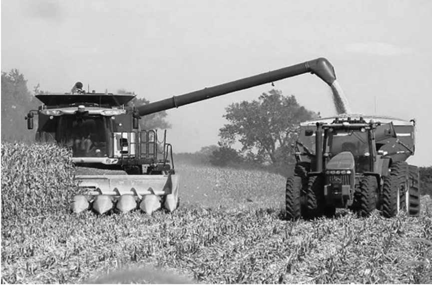
PLATE 2.25 Side view of Autonomous Corn Grain Harvesting System- The Robotic Combine harvester and Grain cart system. Source: Kinze Manufacturers Inc., Williamsburg, Iowa, USA. Note: These are driverless GPS guided vehicles. Their movement in the field is designed by a computer program. The vehicles take shortest and most fuel efficient routes to accomplish the task.
