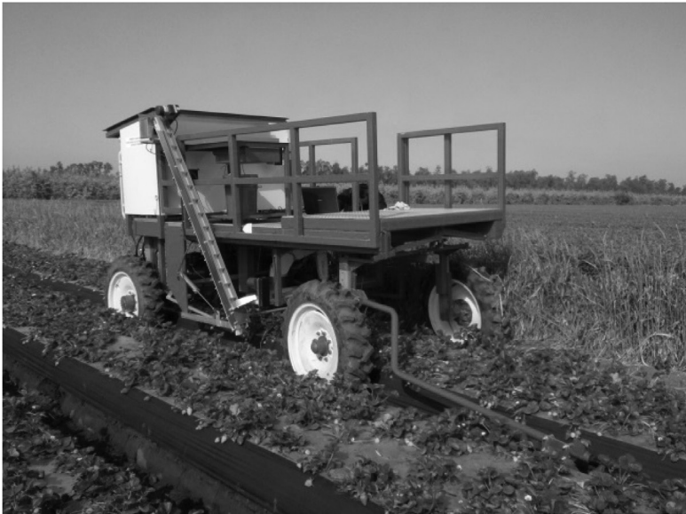
PLATE 2.27 Strawberry Fruit harvesting Robot at work (Top: A robotic arm reaches out to a strawberry fruit using infrared vision, computer decisions and GPS guidance. It is a fairly slow process to pick the fruit, detach it and place it in the cart. Below: A strawberry harvesting robotic combine. This robot is autonomous. It has robotic arms that detach and pick strawberry fruits and place it on a conveyor belt, so that it gets collected into basket/cart. Source: Robotic Harvesting LLC., California, USA).
