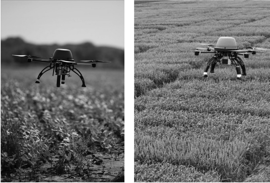
PLATE 3.11 Left: An Agricultural Drone scouting Soybean crop for Pests and Diseases; Right: A venture Quadcopter (Venture Outrider -ProS3/Volt Aerial Robotics) hovering over crop fields. Source: Dr. Rory Paul, Volt Aerial Robotics, Chesterfield, Missouri, USA and United Soybean Board, Iowa. Note: These small, rotary, Agricultural Drones fly at very close height of 10–15 m above the soybean or rice paddy and collect pictures depicting crop health, disease and insect pest attack.).
