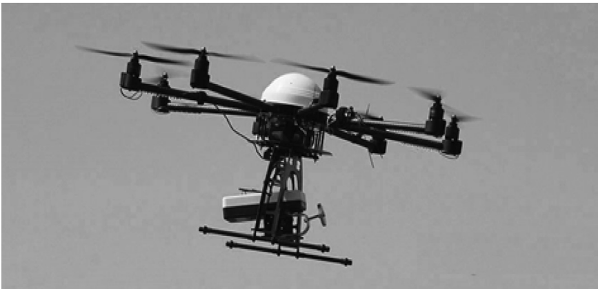
PLATE 3.12A A Hexa-copter drone useful in crop scouting (Source: Dr. Rory Paul, Volt Aerial Robotics, Chesterfield, Missouri, USA).
