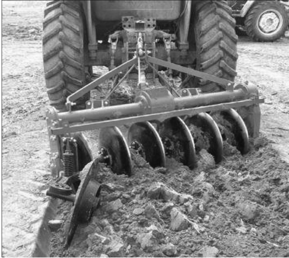
PLATE 2.5 A Disc plow attached to Semi-autonomous Tractor (Source: A Farm near Bangalore, India).
