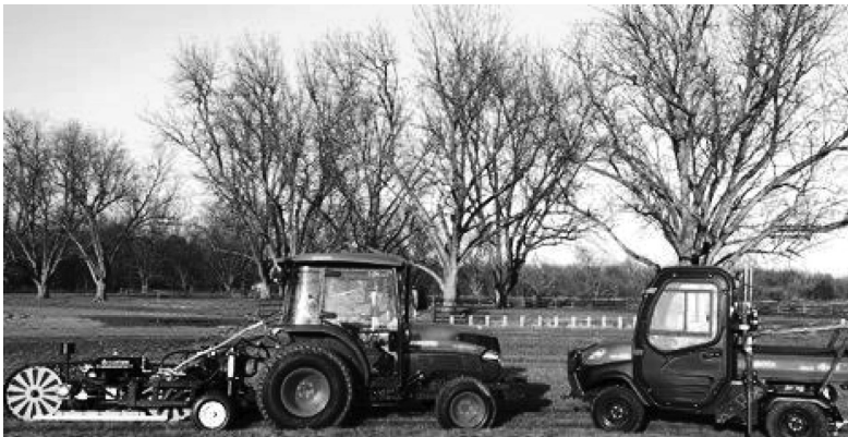
PLATE 4.7 ‘AutoProbe’ (left) and RapidProbe (right) are autonomous soil sampling robots (Source: Drs. Jim and Jeff Burton, AgRobotics, Little Rock, Arkansas, USA; Note: These soil samplers actually dig and extract cores at a rapid rate of 10–20 cores per hr and then prepare a composite a soil sample. They move autonomously based on signals from GPS connectivity. They help farmers in developing soil fertility map).
