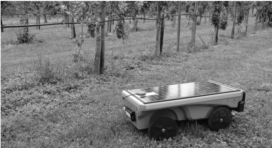
PLATE 2.22 Vitirover – An autonomous robot for weeding fruit plantations of Southern France (Source: Dr. Arnaud Frauchdiere, Vitirover Inc., St de Emilion, France).
