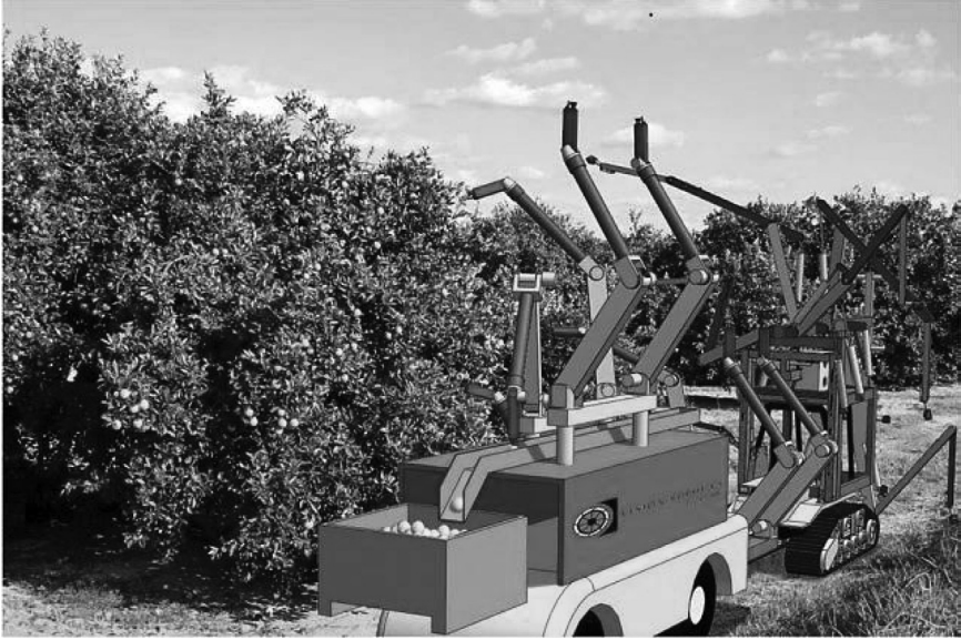
PLATE 2.28 Orange Fruit Picking Robot that operates in the groves (Source: Dr. Tony Koselka, Vision Robotics, San Diego, California, USA).
