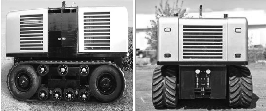
PLATE 2.9 “Spirit” – The Driverless Autonomous Tractor (Source: Mrs. Ann Anderson, Autonomous Tractor Inc., Fargo, North Dakota, USA; Note: The ‘Spirit’ could be attached with variety of implements such as discs, coulter, tines for plowing, harrows for flattening, crushing clods and seed bed preparation. Spirit could also be attached with variable-rate equipment meant for fertilizer, irrigation or pesticide application).
