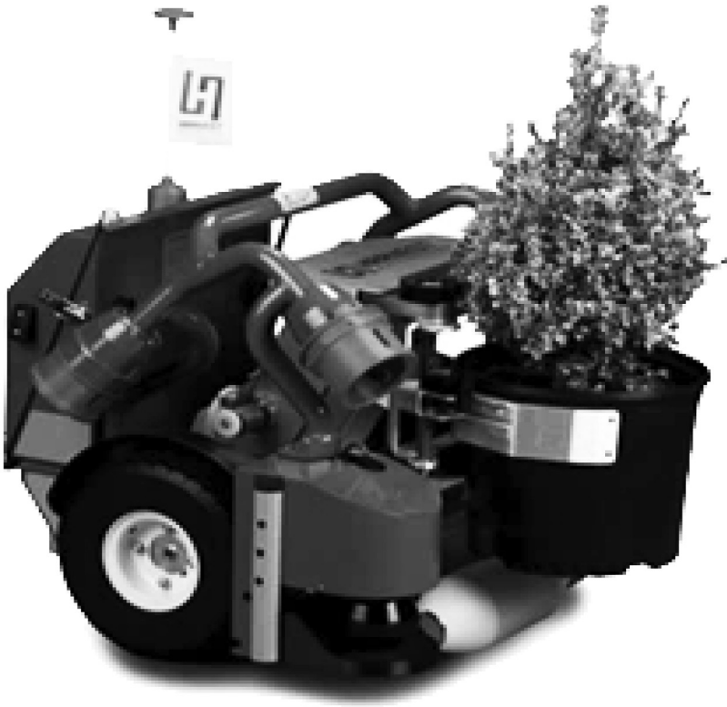
PLATE 2.15 Harvey- the Green House Robot (Model HV-100) (Source: Dr. John Kawola, Harvest Automation Inc., Billerica, Massachusetts, USA; Note: Harvey Robots are already in use in different Nurseries across USA. They are autonomous robots capable of picking, transporting and arranging the pots filled with soil and plants at different stages of growth. They replace hard work and human drudgery in green houses. They are useful while periodic shifting of pots to arrange them at proper spacing).
