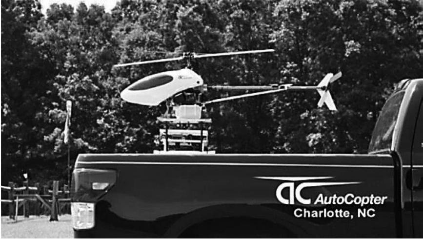
PLATE 3.8A An Autocopter—An agricultural drone (Source: Mr. Donald Effren, President, Autocopter Inc., North Carolina, USA; Note: Autocopters are versatile drones that are gaining in popularity in North American Plains. They are relatively light weight and capable of monitoring, spraying pesticides and applying liquid fertilizer).
