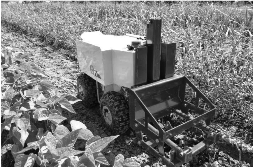
PLATE 2.17 A Small-sized Autonomous Weeder (Source: Dr. Garford, P., Garford Farm machinery, Peterborough, England; www.techdibitis.com ).
