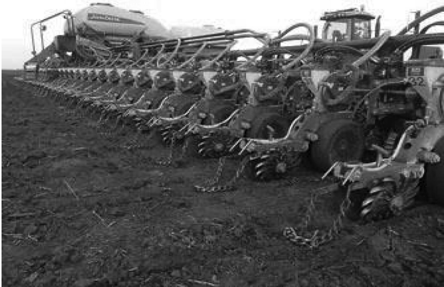
PLATE 2.12 Fertilizer supply to Maize fields Using Semi-Autonomous Tractors and Dispensers [Source: David Nelson, Nelson Farms, Fort Dodge, Iowa, USA; Note: Fertilizer supply to Maize fields (basal dosage) using semi-autonomous tractor and fertilizer-N supply set up. The tractor also has facility for steer less, GPS-aided transit in the field. Fertilizer supply could be regulated using variable-rate applicators. Farmers in the North American Corn belt utilize management zones and Precision Farming approaches to regulate fertilizer-N supply to soil].
