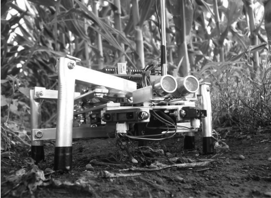
PLATE 2.20 ‘AgAnt’ – An Autonomous robot that inspects the field using Sensors and removes Weeds. AgAnt is small ant-like robot that can work in groups in a field with inter-robot communication (Source: Dr. Tony Grift, Department of Crops Sciences, University of Illinois at Urbana-Champaign, Illinois, USA).
