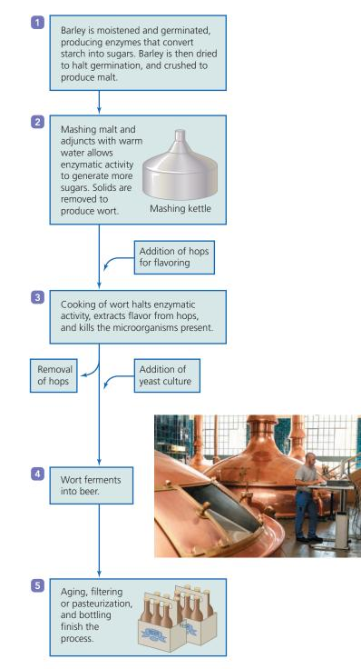
▲ Figure 26.3 The beer-brewing process. The type of beer produced (ale, lager) is determined largely by the type of yeast used (top fermenting or bottom fermenting, respectively).
