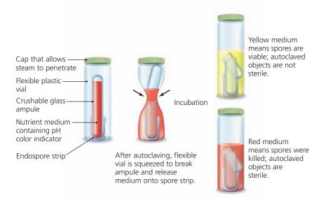
◄ Figure 9.8 Sterility indicators. A commercial endospore-test ampule, which is included among objects to be sterilized. After autoclaving is complete, the medium, which contains a pH color indicator, is released onto the endospore strip when the ampule is broken. If the endospores are still alive, their metabolic wastes lower the pH, changing the color of the medium.
