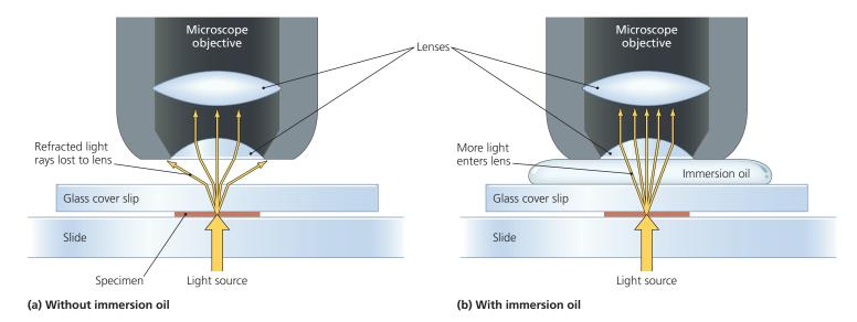
▲ Figure 4.5 The effect of immersion oil on resolution. (a) Without immersion oil, light is refracted as it moves from the cover glass into the air. Part of the scattered light misses the objective lens. (b) With immersion oil. Because light travels through the oil at the same speed as it does through glass, no light is refracted as it leaves the specimen and more light enters the lens, which increases resolution.
