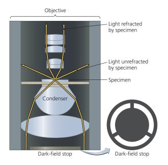
▲ Figure 4.6 The light path in a dark-field microscope. A dark-field stop prevents light from entering the specimen directly; only light rays that are scattered by the specimen reach the objective lens and can be seen. The resulting high-contrast image—a brightly lit specimen against a dark background—enhances resolution.
