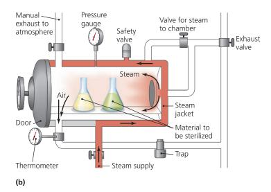
▲ Figure 9.7 An autoclave. (a) A photo of a laboratory autoclave. (b) A schematic of an autoclave, showing how it functions.
