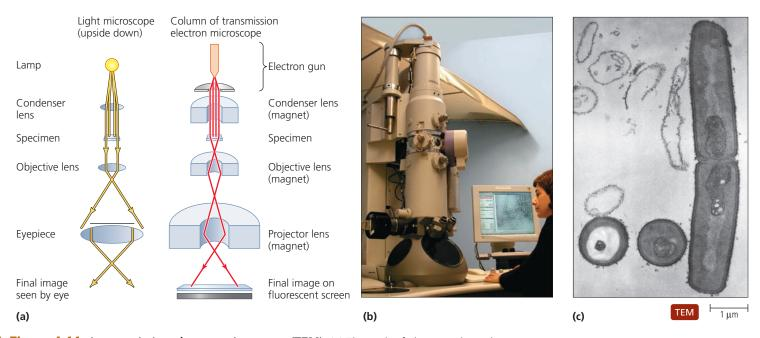
▲ Figure 4.11 A transmission electron microscope (TEM). (a) The path of electrons through a TEM, as compared to the path of light through a light microscope (at left, drawn upside down to facilitate the comparison). (b) TEMs are much larger than light microscopes. (c) Transmission electron image of a bacterium, *Bacillus subtilis*. A transmission electron micrograph reveals much internal detail not visible by light microscopy. Why must air be evacuated from the column of an electron microscope?
