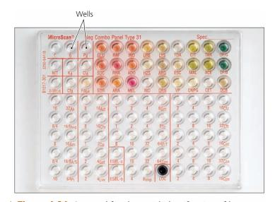
▲ Figure 4.24 One tool for the rapid identification of bacteria, the automated MicroScan system. A MicroScan panel, a plate containing numerous wells, each the site of a particular biochemical test. The instrument ascertains the identity of the organism by reading the pattern of colors in the wells after the biochemical tests have been performed.
