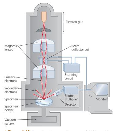
▲ Figure 4.12 Scanning electron microscope (SEM). The SEM uses magnetic lenses to focus a beam of primary electrons, which are scanned across the metal-coated surface of a specimen. Secondary electrons, knocked off the surface of the specimen by the primary electrons, are collected by a detector, and their signal is amplified and displayed on a monitor.
