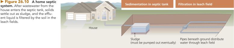
system. After wastewater from the house enters the septic tank, solids settle out as sludge, and the effluent liquid is filtered by the soil in the leach fields.
