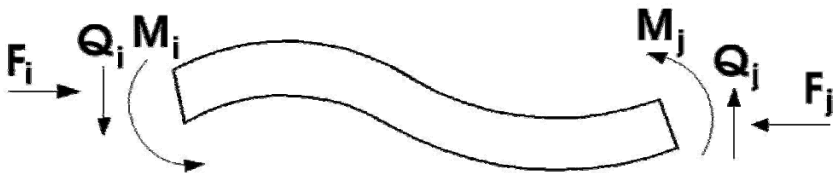
Fig. 4.1 Shear and normal forces and moments acting on the beam element (van Mier et al. 1995)
