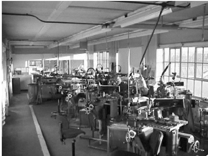
Figure 2.57 A 1930s machine shop in Sheffield which made use of night ventilation to cool the concrete and brick structure and thus reduce the frequency of overheating
