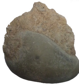
Figure 2. Configuration of a typical RA from previous demolition.
