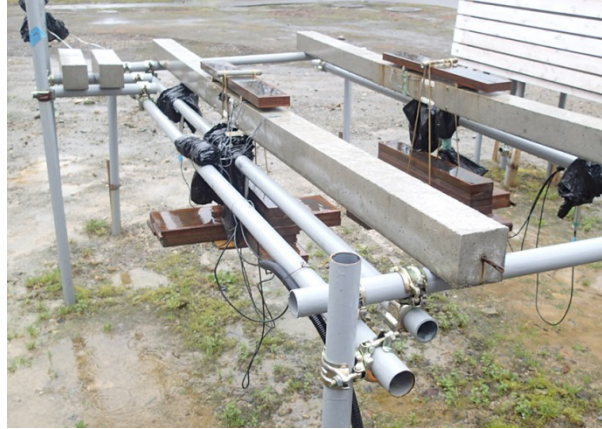
Figure 6. Sustaining loading test of PC beam under natural environment.
