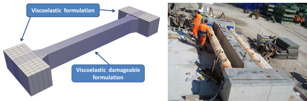
Figure 1. Experimental specimen (right) and finite elements mesh (left), Reprinted from Simoni and Schrefler (2014), Copyright (2014), with permission from Elsevier.
