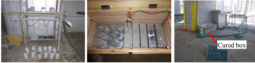
(a) Rain-d specimens (b) No-rained, sealed specimens. (c) View. Figure 4. Specimens cured near the PC girder.
