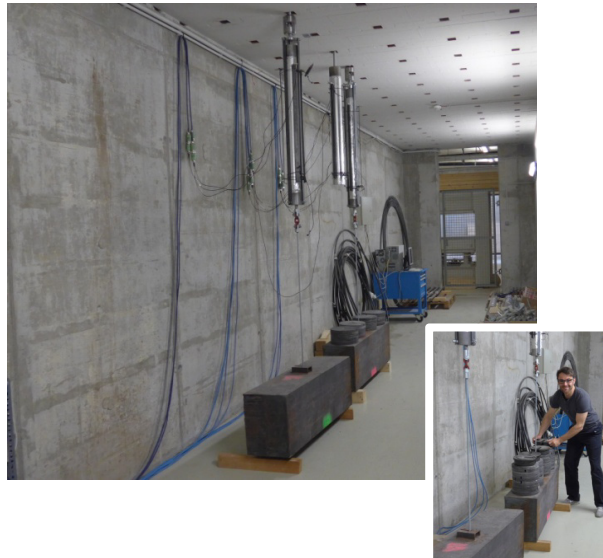
Figure 5. Hanging cylindrical specimens with suspended load for tensile creep monitoring under changing stress level.
