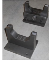
Figure 3. New EMM-ARM steel supports.
