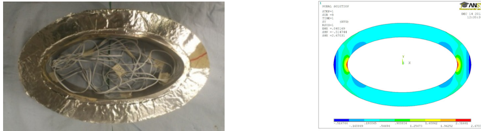
(a) crack position (b) circumferential stress contour at 11 th day
