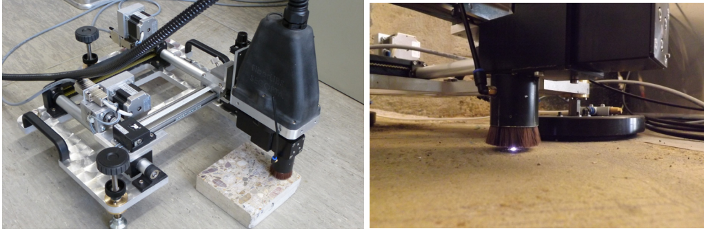
Figure 1. Right: Translation stage with measuring head and a core cut in the middle to do measurements on the cross section. During the measurement the head is moved line by line in a plane parallel to the sample surface. Left: Detailed view – showing the plasma on the sample surface
