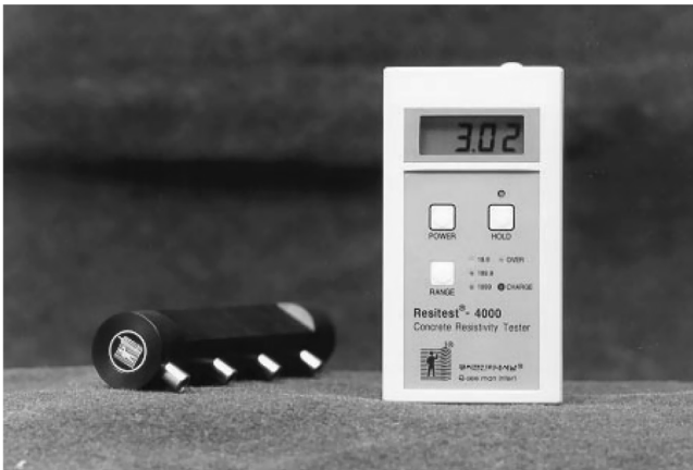
FIGURE 4.28 Electrical resistivity measurement equipment.
