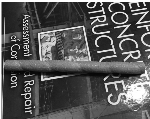
FIGURE 7.4 Shape of the reinforcement bar from GFRP.
