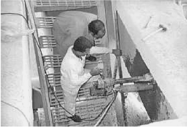
FIGURE 4.5 How to take a core sample.
