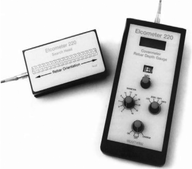
FIGURE 4.23 Concrete cover thickness measurement machine.
