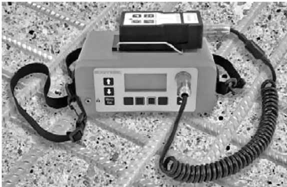
FIGURE 5.3 Electromagnetic cover meter.
