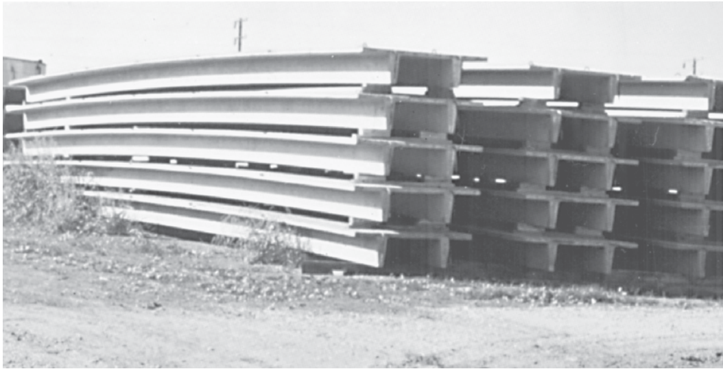
FIGURE 18.8. Precast, Prestressed Concrete Members at Casting Yard.
