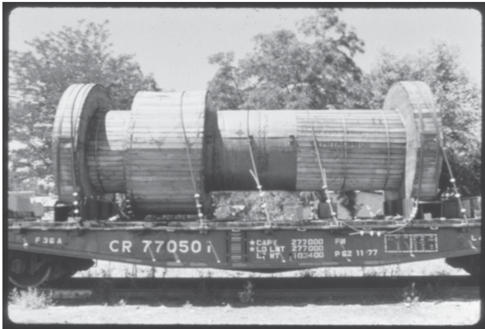
FIGURE 4.18. Claims-Defense Photo of 150-Ton Turbine-Generator Shaft as It Arrived at the End of the Rail Line Prior to Release to Contractor for Transport to Project Site.
