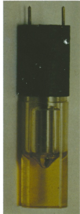
Fig. 26. Large-scale production of fused cells. In principle the helical chamber consists of a hollow Perspex tube around which are wound two cylindrical Pt-electrodes at a distance of, say, 200\ \mu\text{m} (total length about 1 m). The Perspex tube can be filled with cooling medium in order to avoid temperature increases during the field application. The Perspex tube with the Pt wires is introduced into a cylindrical jacket which already contains the cell suspension. The cell suspension rises up through the intervening space. Analogous to the arrangement in Figs. 19, 20 and 25, cell chains are formed between the parallel electrode wires in response to an alternating field. After application of a breakdown pulse and subsequent fusion, the cells can be collected by centrifugation into a receptacle by way of a valve. The receptacle is disposable and can very easily be removed for cloning of the fused hybrids. The whole procedure can be performed under sterile conditions. From (67); the photograph was given by courtesy of GCA Corporation, Chicago, Illinois, USA
