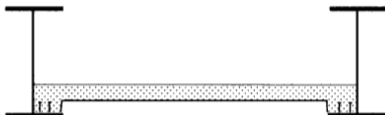
Fig. 6.12. Example of a composite beam with the slab in tension at mid-span
