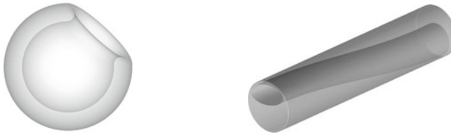
Fig. 1: Translucent view of the spherical cavity and the Channel air intake used for the tests
