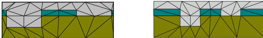
Fig. 2: Topologically equivalent grids which can be mapped by piecewise linear transformation onto each other
