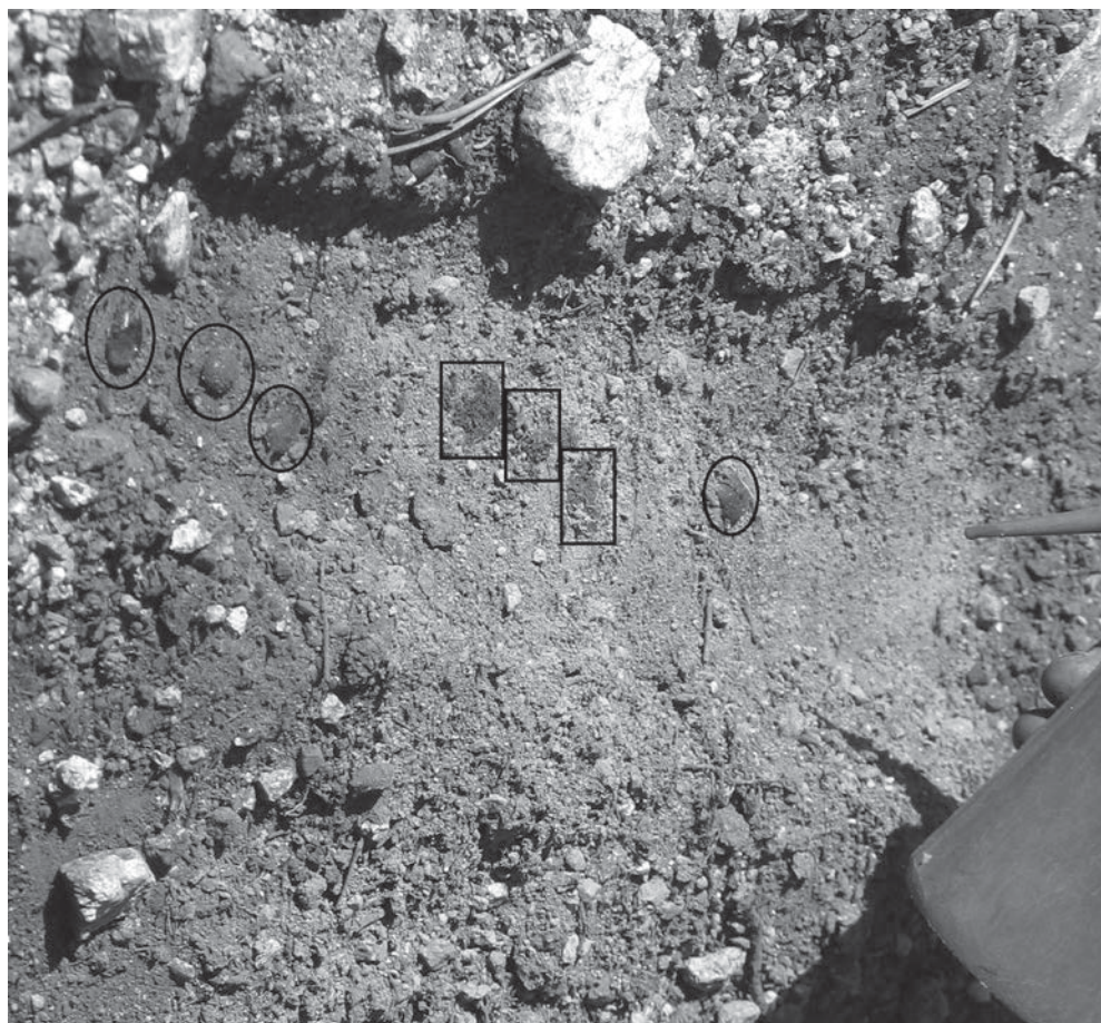
Fig. 13.1. Water-repellent soil conditions after a wildfire and a 30-minute rainfall event showing saturated surface soil and dry soil a few centimetres below the surface. Circles indicate water drops on the soil surface, rectangles indicate water drops that have infiltrated.
